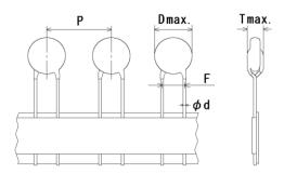
Note) The mark '\*' of Lead Style differ from lead spacing (F), lead diameter (d) and pitch of component (P). Please see the following list or taping specification about details.
