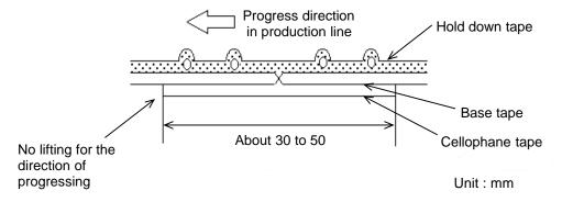
b) When hold down tape is spliced
