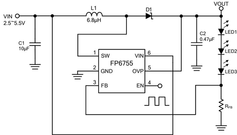
Figure 2. Typical Application Circuit of FP6755 SOT-23-6 Package
