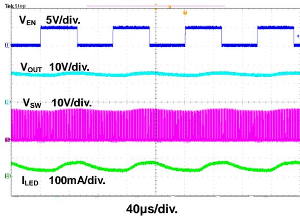
Figure 8. PWM Dimming Response Waveforms at a Frequency of 10kHz
