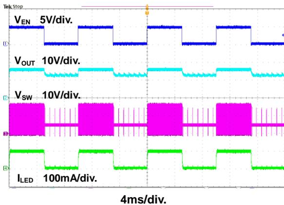
Figure 9. PWM Dimming Response Waveform at a Frequency of 100Hz
