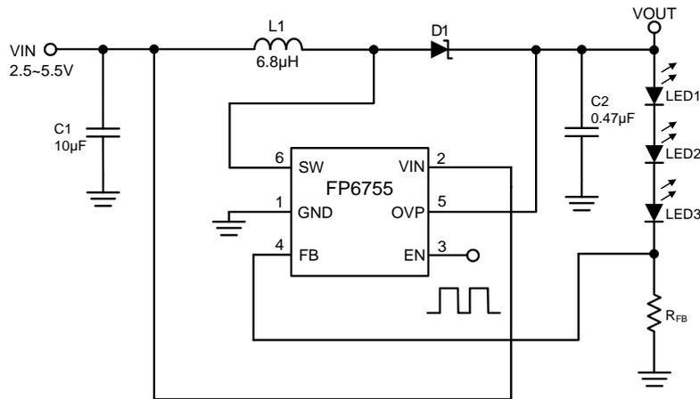
Figure 3. Typical Application Circuit of FP6755 TDFN-6 (2mmx2mm) Package
