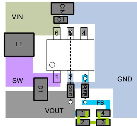
Figure 16. Layout Diagram
