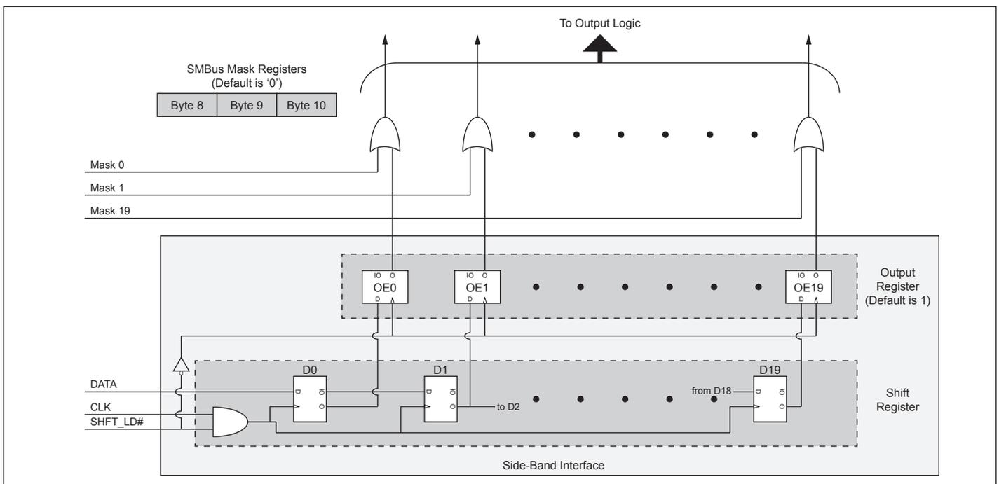
**Figure 1. Side Band Interface Control Logic Description**
