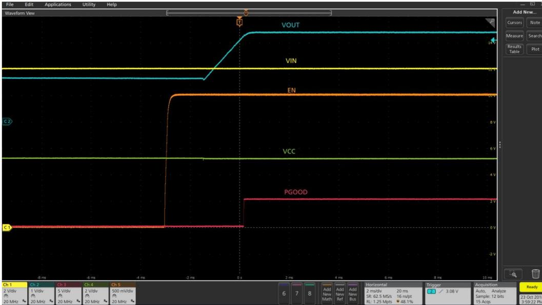
**Figure 21 Startup into pre-bias (Ch1:PV<sub>IN</sub>, Ch2: V<sub>OUT</sub>, Ch3: PGood, Ch4:V<sub>CC</sub>, Ch5: Enable)**
