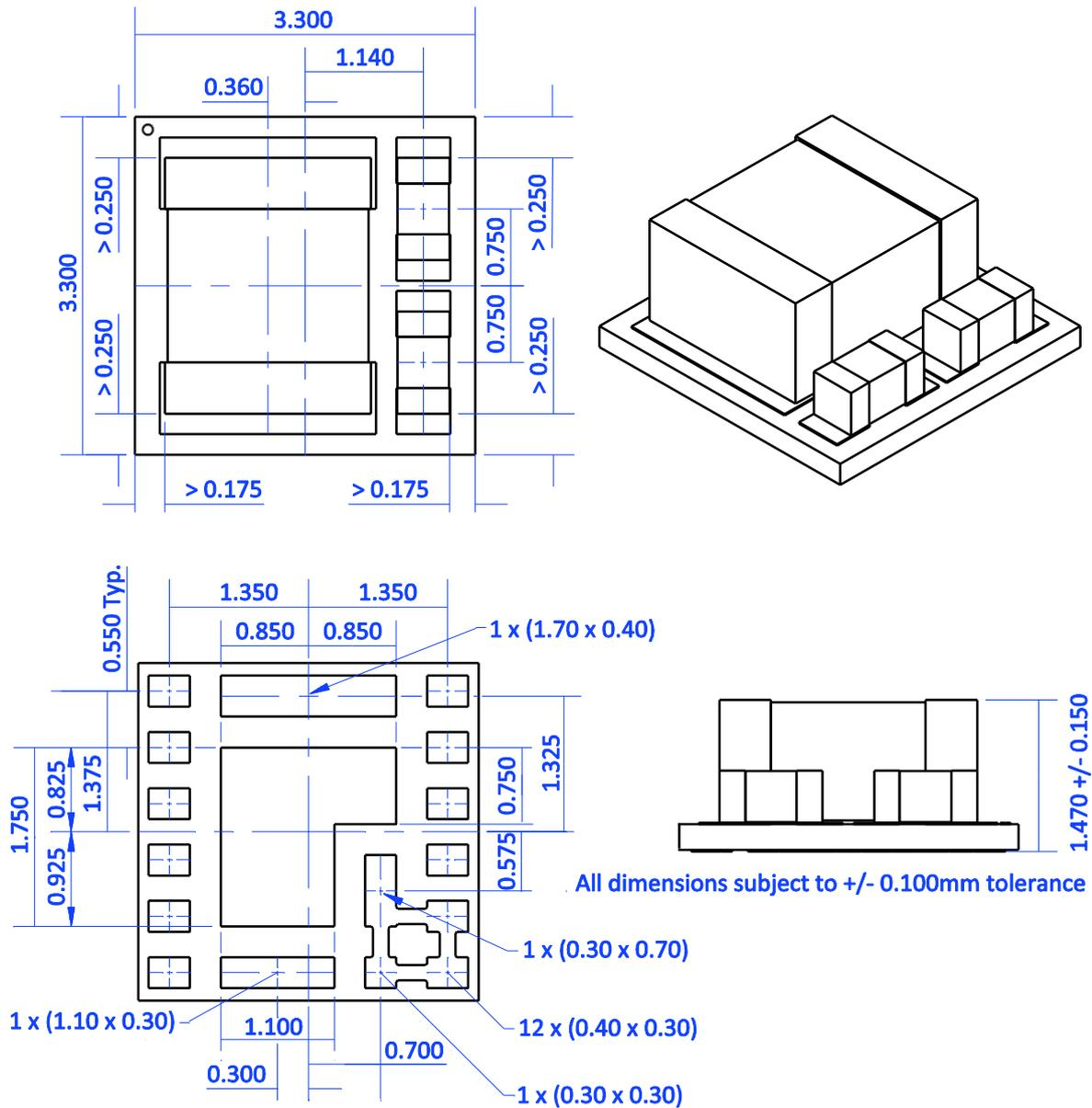
Figure 31 Dimensioned drawings
