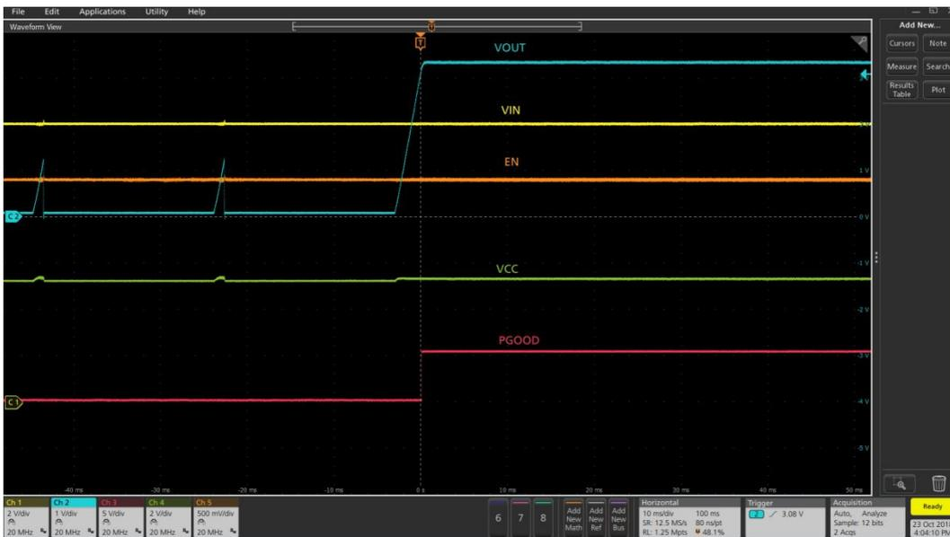
**Figure 22 Over-current protection and auto-recover to 4A (Ch1:PV<sub>IN</sub>, Ch2: V<sub>OUT</sub>, Ch3: PGood, Ch4:V<sub>CC</sub>, Ch5: Enable)**
