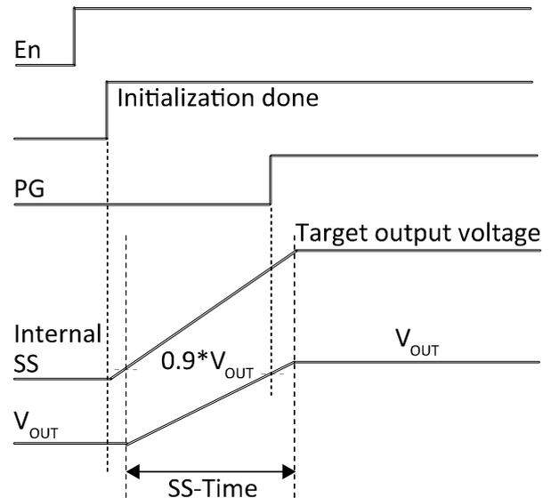
**Figure 8** Theoretical operational waveforms during soft-start
