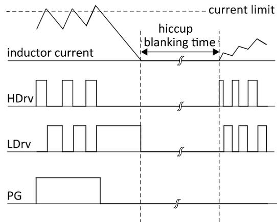
Figure 12 Illustration of OCP in hiccup mode
