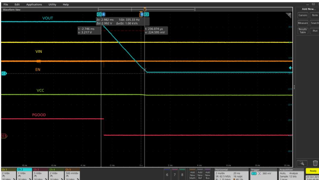
**Figure 20 Soft turn off at 4A load (Ch1:PV<sub>IN</sub>, Ch2: V<sub>OUT</sub>, Ch3: PGood, Ch4:V<sub>CC</sub>, Ch5: Enable)**
