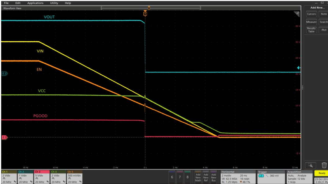
**Figure 19 Shutdown with Enable de-assertion at 4A load**
