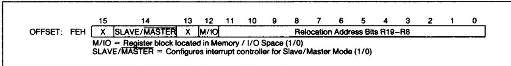
Figure 9. Relocation Register
