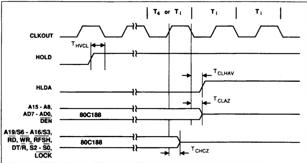
HOLD/HLDA WAVEFORMS (Leaving Hold)
