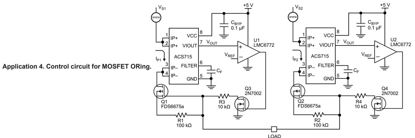
Application 4. Control circuit for MOSFET Oring.
