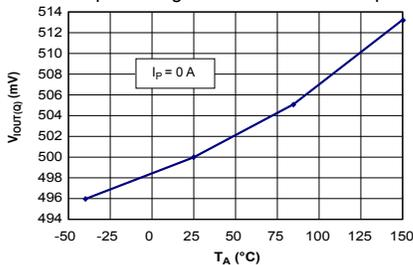
0 A Output Voltage Current versus Ambient Temperature
