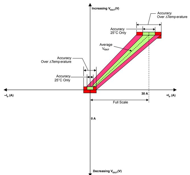
**Figure 1: Output Voltage versus Sampled Current**
