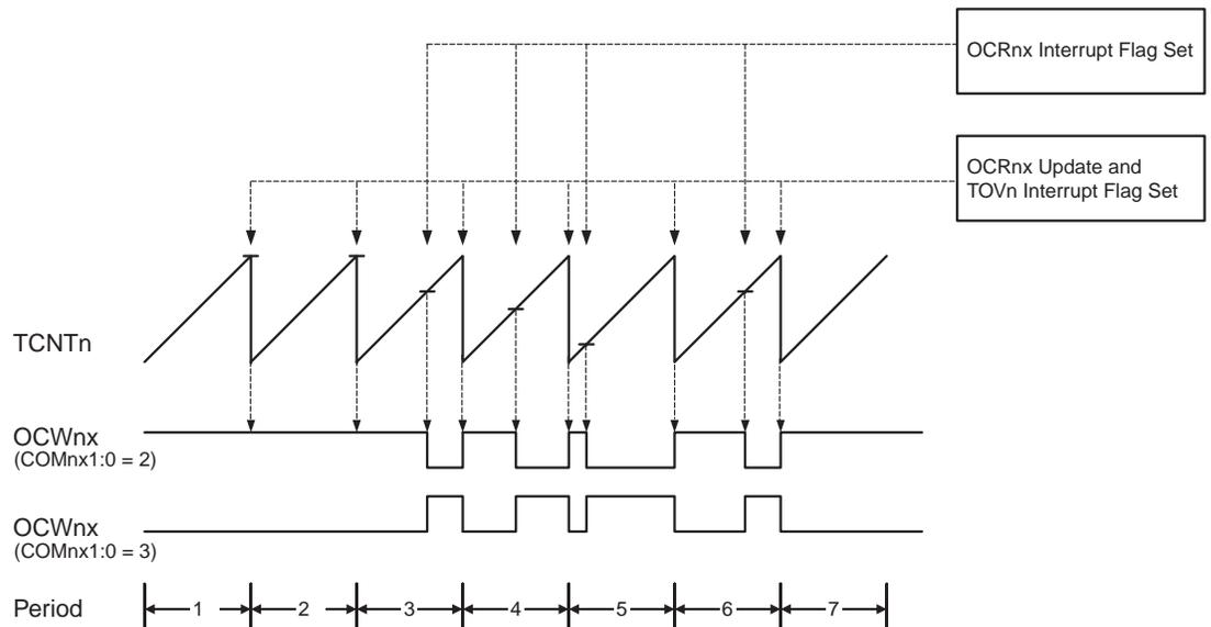
The Timer/Counter Overflow Flag (TOV1) is set each time the counter reaches TOP. If the interrupt is enabled, the interrupt handler routine can be used for updating the compare value.
