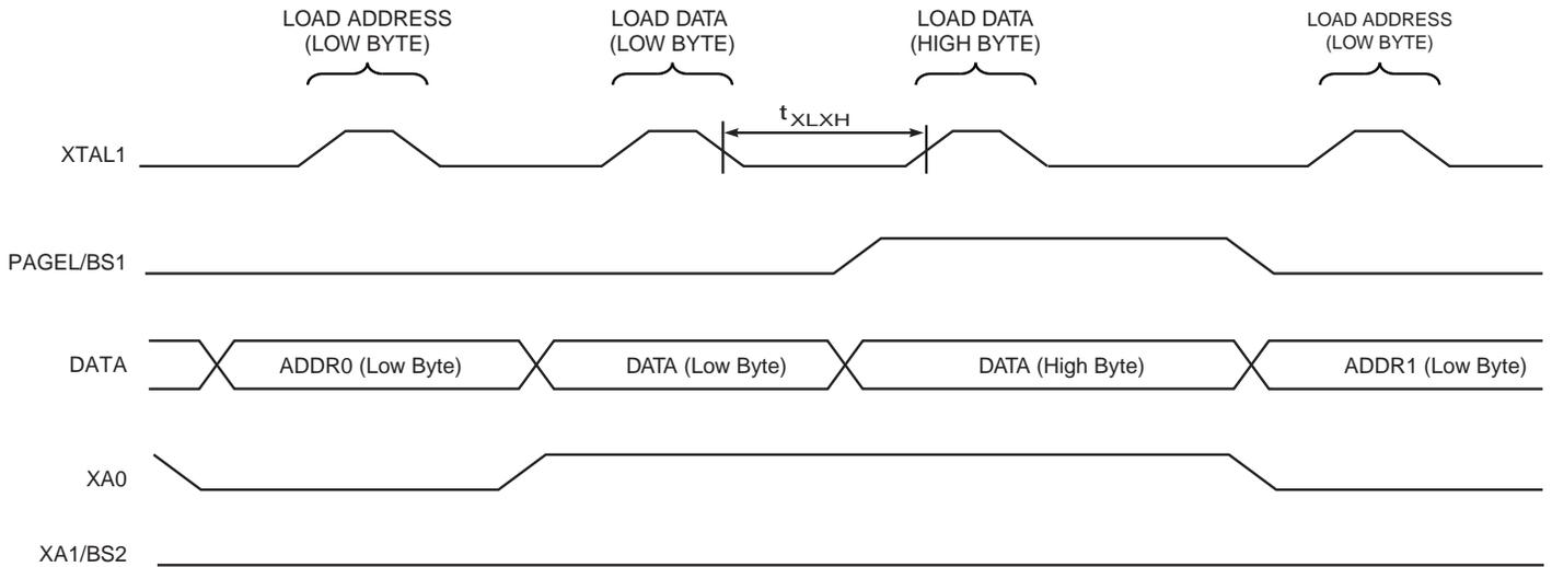
Note: The timing requirements shown in [Figure 19-5](#) (i.e.,  $t_{DVXH}$ ,  $t_{XHL}$ , and  $t_{XLDX}$ ) also apply to loading operation.
