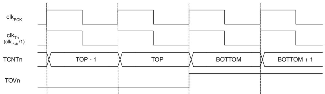
Figure 12-16 shows the same timing data, but with the prescaler enabled, in all modes other than Phase and Frequency Correct PWM Mode.
