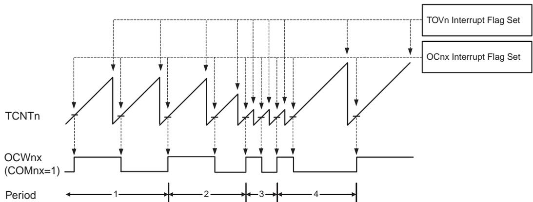
The counter value (TCNT1) that is shown as a histogram in [Figure 12-11](#) is incremented until the counter value matches the TOP value. The counter is then cleared at the following clock cycle. The diagram includes the Waveform Output (OCW1x) in toggle Compare Mode. The small horizontal line marks on the TCNT1 slopes represent Compare Matches between OCR1x and TCNT1.
