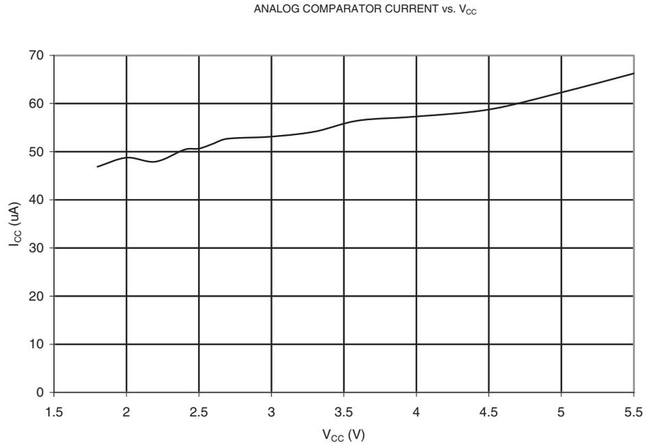
**Figure 20-67.** ADC Current vs.  $V_{CC}$  (AREF =  $AV_{CC}$ )
