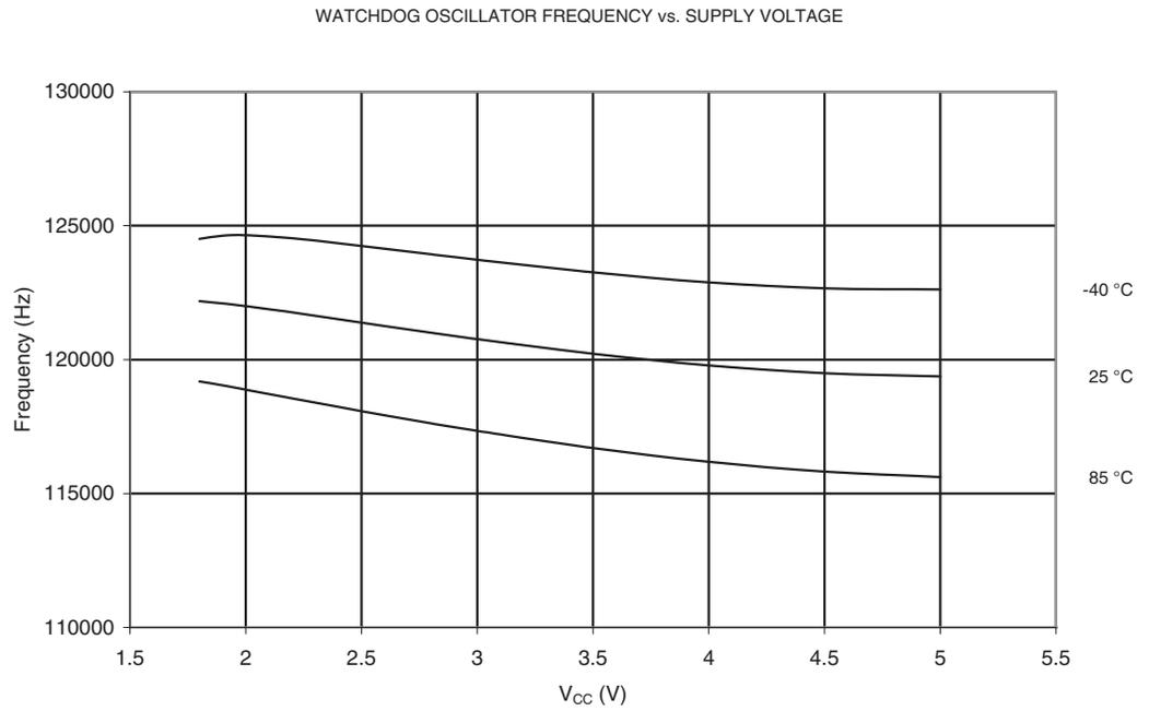
**Figure 20-48.** Frequency of Watchdog Oscillator vs. Temperature
