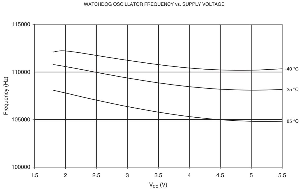
**Figure 20-150.** Frequency of Watchdog Oscillator vs. Temperature
