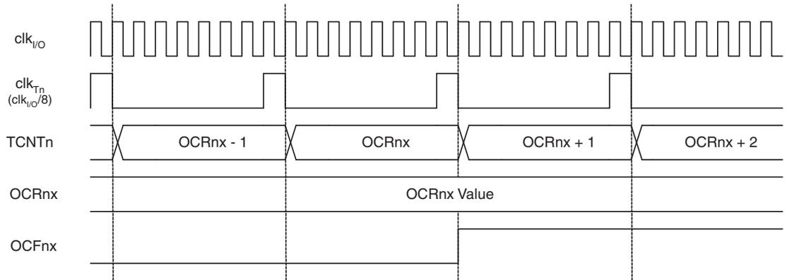
Figure 11-10 shows the setting of OCF0A and the clearing of TCNT0 in CTC mode.
