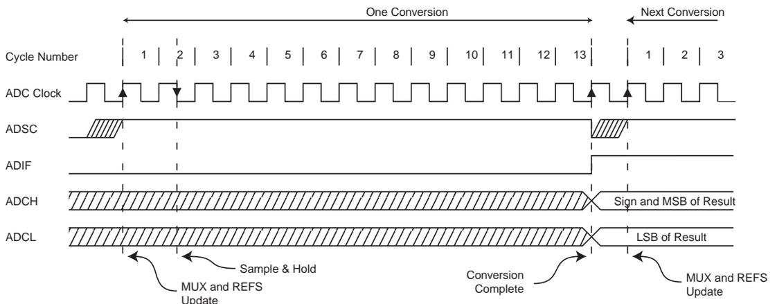
When Auto Triggering is used, the prescaler is reset when the trigger event occurs. See [Figure 15-6](#). This assures a fixed delay from the trigger event to the start of conversion. In this mode, the sample-and-hold takes place two ADC clock cycles after the rising edge on the trigger source signal. Three additional CPU clock cycles are used for synchronization logic.
