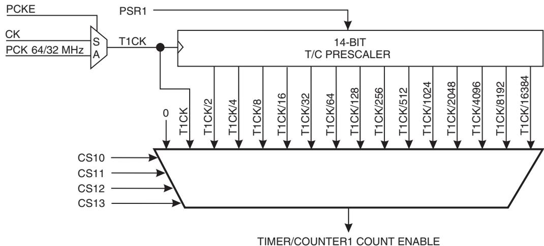
In the asynchronous clocking mode the clock selections are from PCK to PCK/16384 and stop, and in the synchronous clocking mode the clock selections are from CK to CK/16384 and stop. The clock options are illustrated in [Figure 12-3](#) and described in “[TCCR1B – Timer/Counter1 Control Register B](#)” on [page 113](#).
