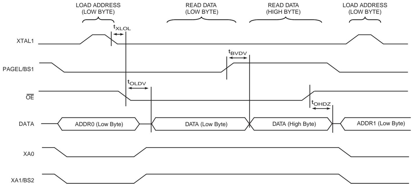
Note: The timing requirements shown in Figure 19-5 (i.e.,  $t_{DVXH}$ ,  $t_{XHXL}$ , and  $t_{XLDX}$ ) also apply to reading operation.
