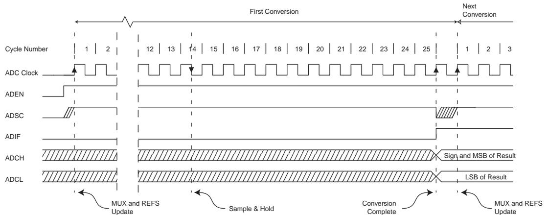
The actual sample-and-hold takes place 1.5 ADC clock cycles after the start of a normal conversion and 13.5 ADC clock cycles after the start of an first conversion. See [Figure 15-5](#).
