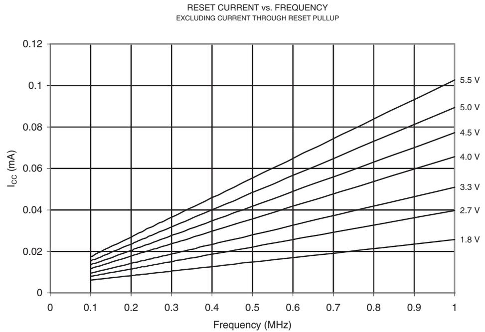
**Figure 20-116.** Reset Supply Current vs. Frequency (1 - 20 MHz, Excluding Current Through the Reset Pull-up)
