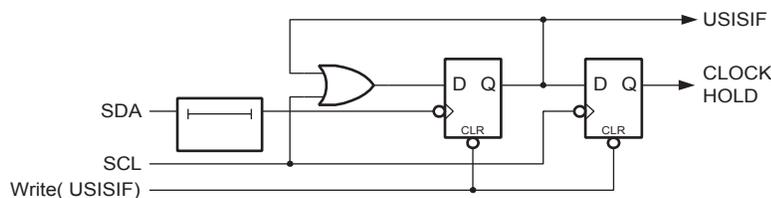
The start condition detector works asynchronously and can therefore wake up the processor from power-down sleep mode. However, the protocol used might have restrictions on the SCL hold time. Therefore, when using this feature in this case the Oscillator start-up time set by the CKSEL Fuses (see [“Clock System” on page 24](#)) must also be taken into the consideration. Refer to the USISIF bit description on page 131 for further details.
