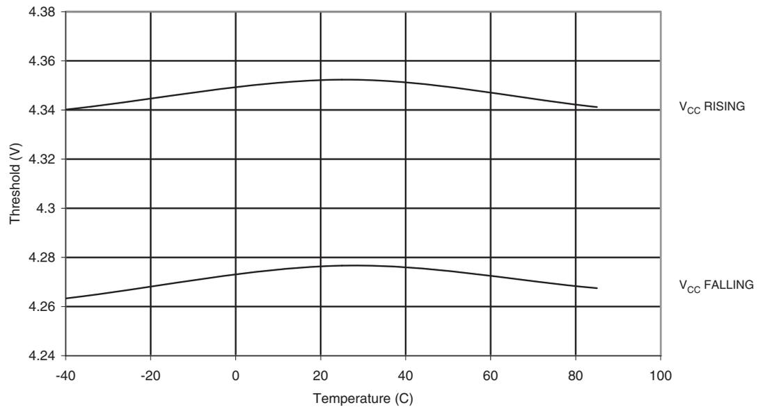
**Figure 20-43.** BOD Threshold vs. Temperature (BOD Level set to 2.7V)
