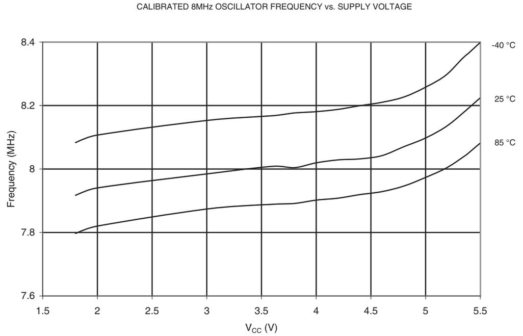
**Figure 20-152.** Frequency of Calibrated 8.0 MHz Oscillator vs. Temperature
