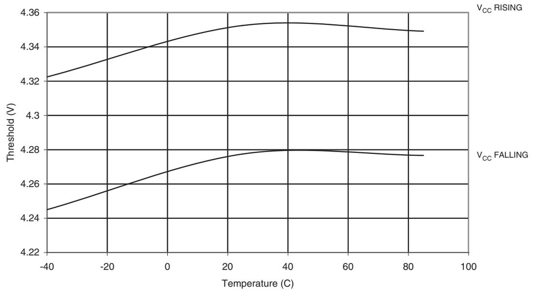
**Figure 20-145.**BOD Threshold vs. Temperature (BOD Level set to 2.7V)
