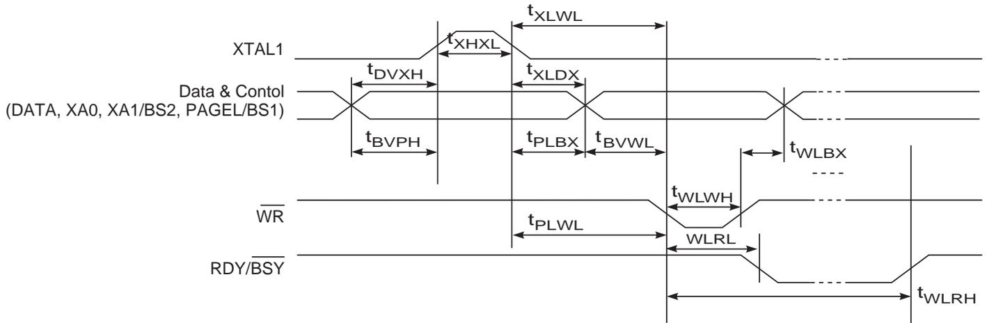
**Figure 19-6.** Parallel Programming Timing, Loading Sequence with Timing Requirements
