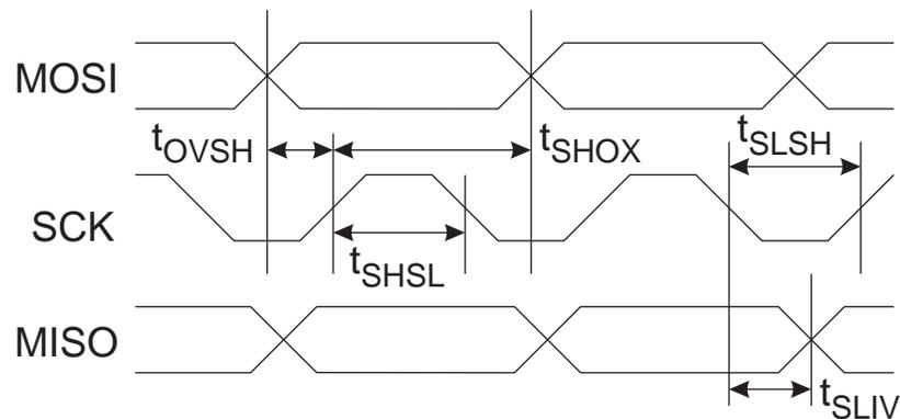
**Table 19-8.** Serial Programming Characteristics,  $T_A = -40^{\circ}\text{C}$  to  $85^{\circ}\text{C}$ ,  $V_{CC} = 1.8 - 5.5\text{V}$  (Unless Otherwise Noted)
