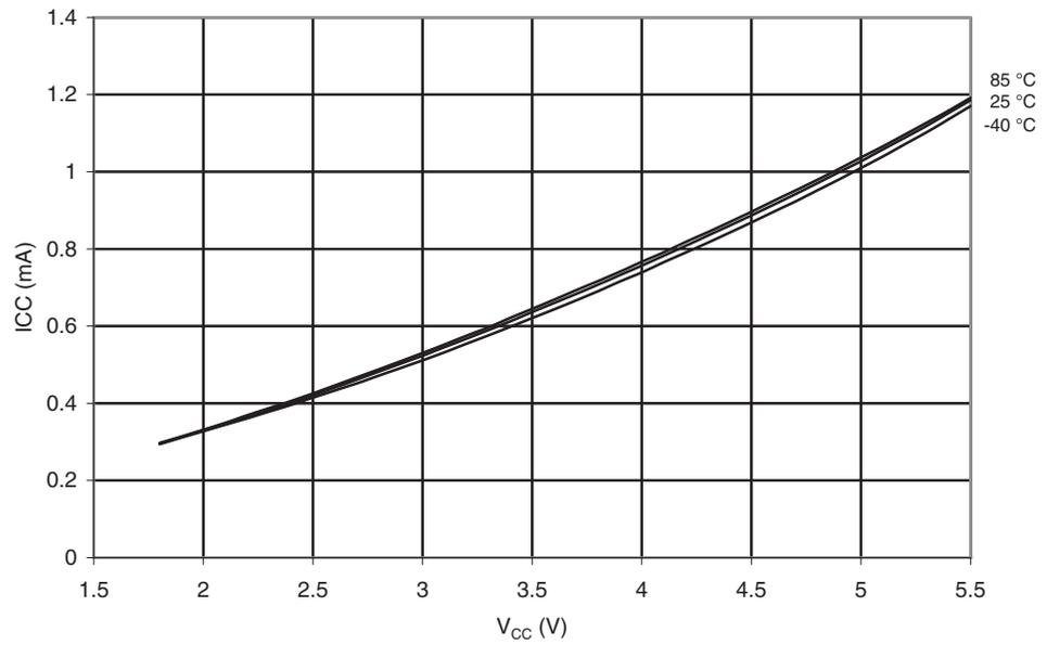
**Figure 20-9.** Idle Supply Current vs.  $V_{CC}$  (Internal Calibrated Oscillator, 1 MHz)
