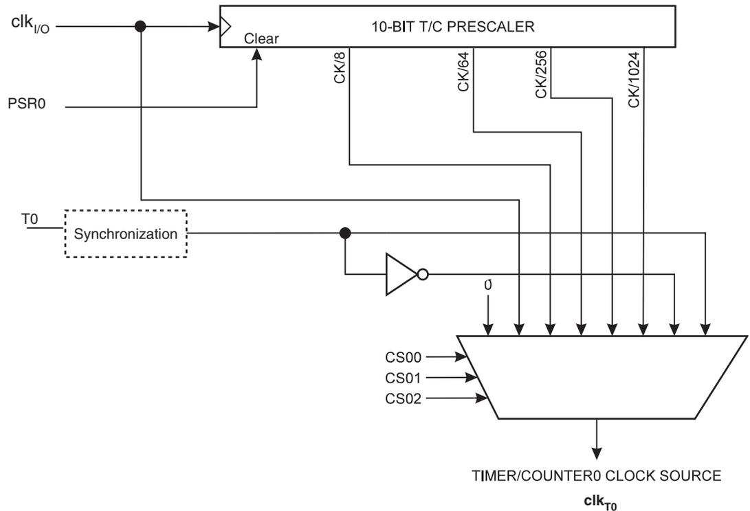
Note: 1. The synchronization logic on the input pins (T0) is shown in [Figure 11-3](#).
