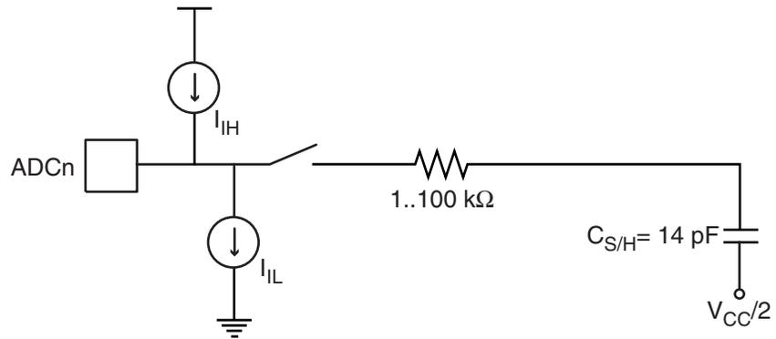
The capacitor in [Figure 15-8](#) depicts the total capacitance, including the sample/hold capacitor and any stray or parasitic capacitance inside the device. The value given is worst case.
