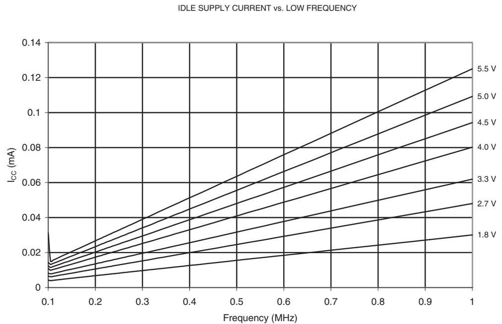
**Figure 20-7.** Idle Supply Current vs. Frequency (1 - 20 MHz)
