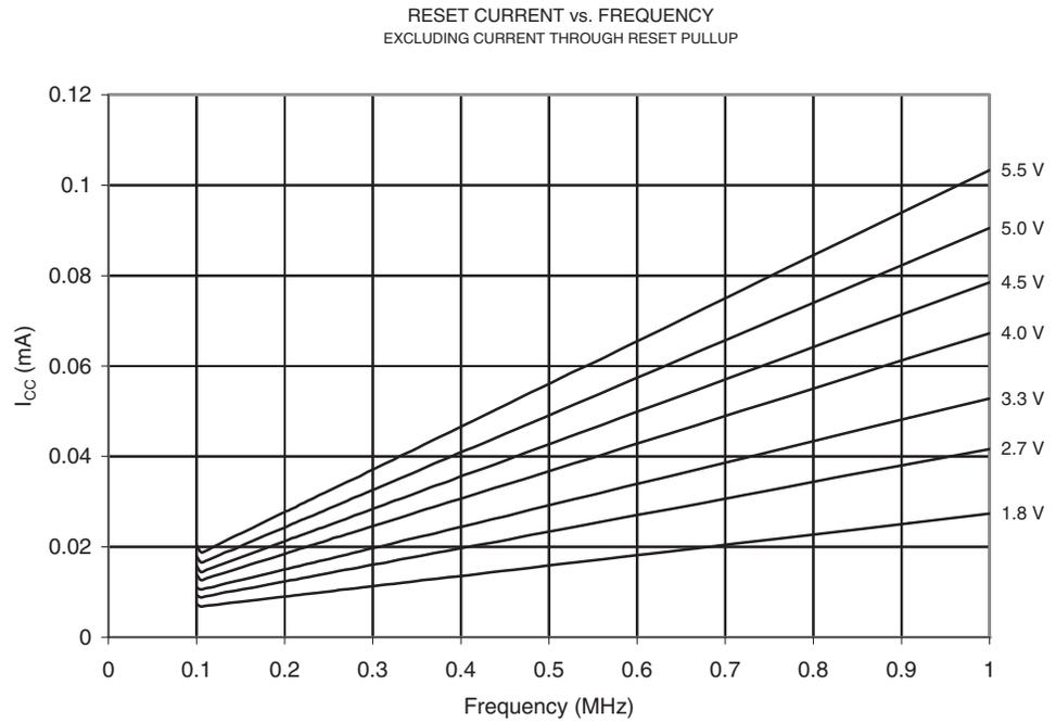
**Figure 20-14.** Reset Supply Current vs. Frequency (1 - 20 MHz, Excluding Current Through the Reset Pull-up)
