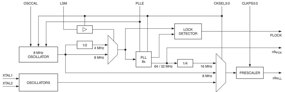
The internal PLL is enabled when CKSEL fuse bits are programmed to '0001' and the PLLE bit of PLLCSR is set. The internal oscillator and the PLL are switched off in power down and stand-by sleep modes.
