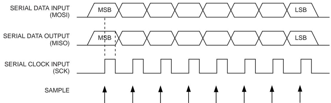
**Figure 19-4.** Serial Programming Timing
