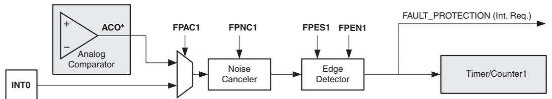
Fault Protection mode is enabled by setting the Fault Protection Enable (FPEN1) bit and triggered by a change in logic level at external interrupt pin (INT0). Alternatively, fault protection mode can be triggered by the Analog Comparator Output (ACO).
