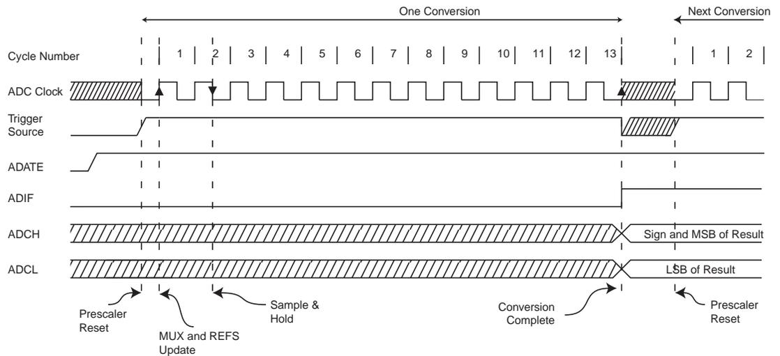
In Free Running mode (see [Figure 15-7](#)), a new conversion will be started immediately after the conversion completes, while ADSC remains high.
