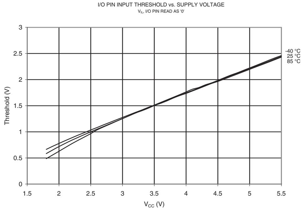
**Figure 20-89.**  $V_{IH}-V_{IL}$ : Input Hysteresis vs.  $V_{CC}$  (I/O Pin)
