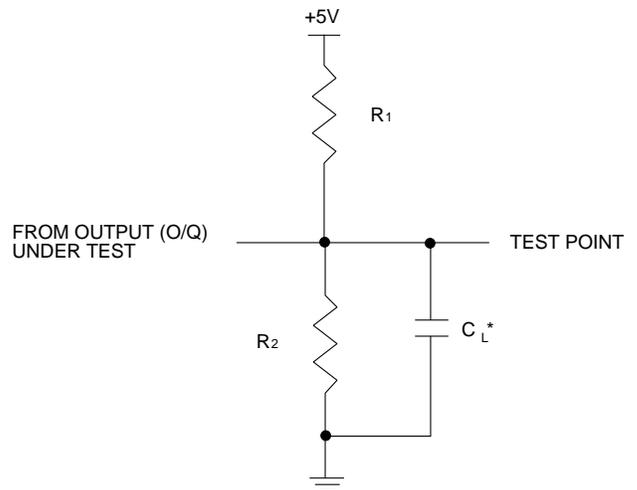
\*C<sub>L</sub> INCLUDES TEST FIXTURE AND PROBE CAPACITANCE
