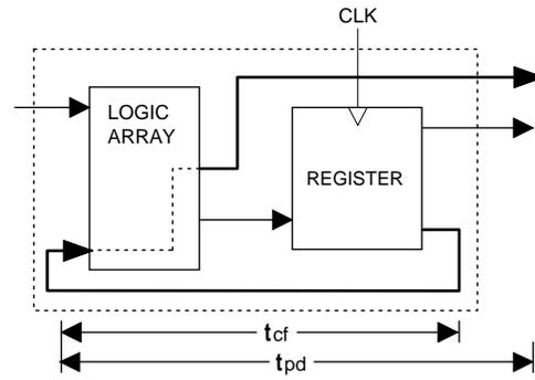
**f<sub>max</sub> with Internal Feedback 1/(t<sub>su</sub>+t<sub>cf</sub>)**
