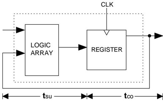
**f<sub>max</sub> with External Feedback 1/(t<sub>su</sub>+t<sub>co</sub>)**
