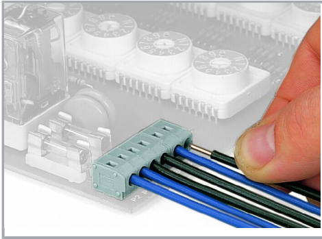
Inserting a solid conductor via push-in termination.
