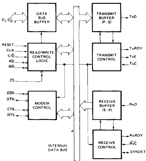
Figure 1. Block Diagram
