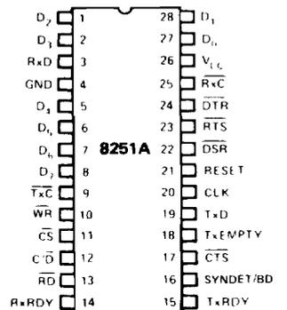
Figure 2. Pin Configuration
