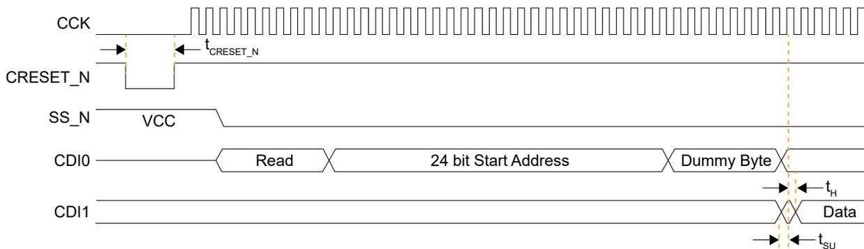
Figure 32: SPI Passive Mode (x1) Timing Sequence
