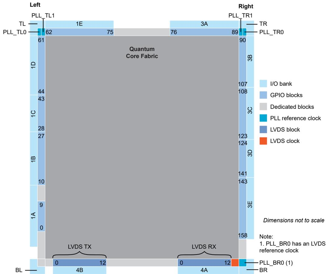
Figure 38: Floorplan Diagram for FPGAs in BGA324 Packages (with DDR and MIPI)
