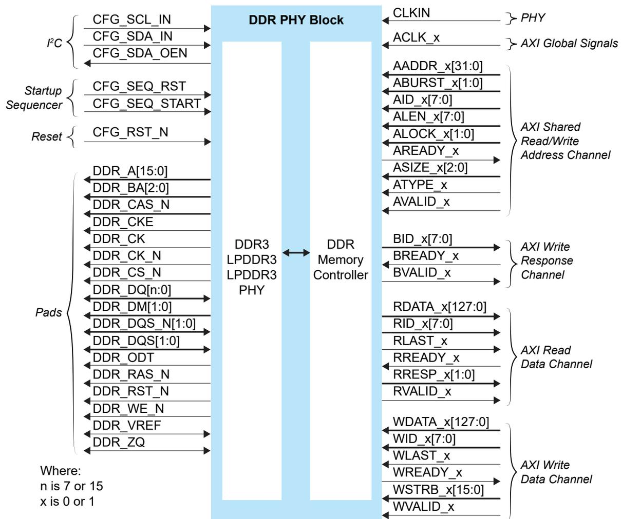
The DDR DRAM block supports an I<sup>2</sup>C calibration bus that can read/write the DDR configuration registers. You can use this bus to fine tune the DDR PHY for high performance.
