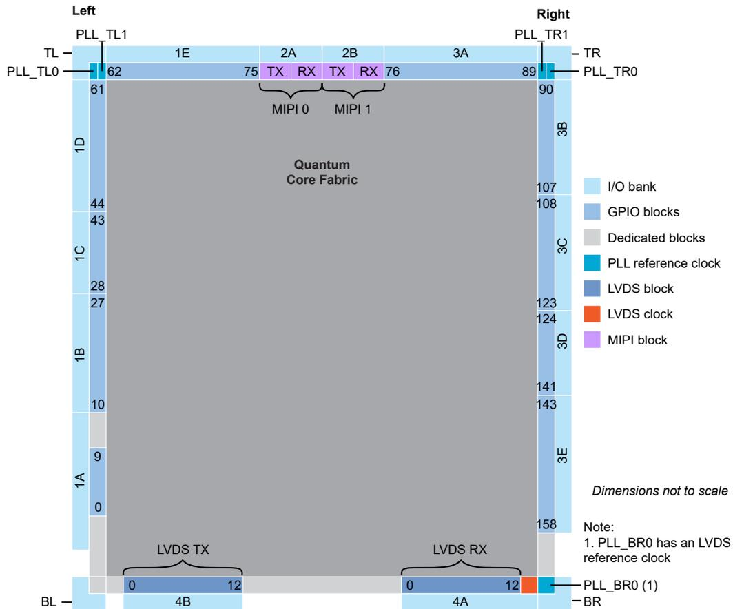
Figure 37: Floorplan Diagram for FPGAs in BGA256 Packages
