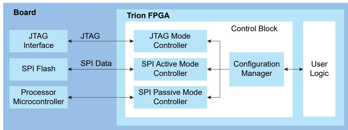
In active mode, the FPGA controls the configuration process. An oscillator circuit within the FPGA provides the configuration clock. The bitstream is typically stored in an external serial flash device, which provides the bitstream when the FPGA requests it.
