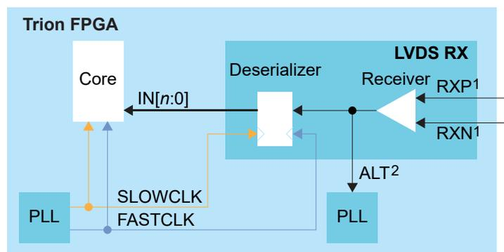
1. There is a  $\sim 30k \Omega$  internal weak pull-up to VCCIO (3.3V).
