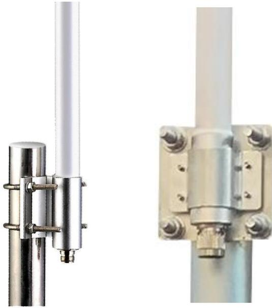
For correct mast/pole assembly, the metallic support must fully contact the metallic antenna support sleeve, not the fiber glass body.
