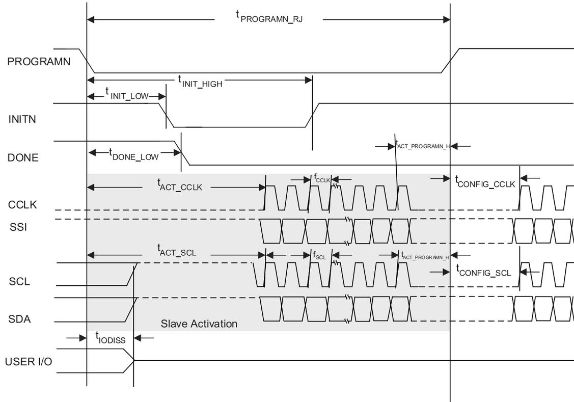
Figure 3.17. Slave SPI/I<sup>2</sup>C/I<sup>3</sup>C PROGRAMN Timing
