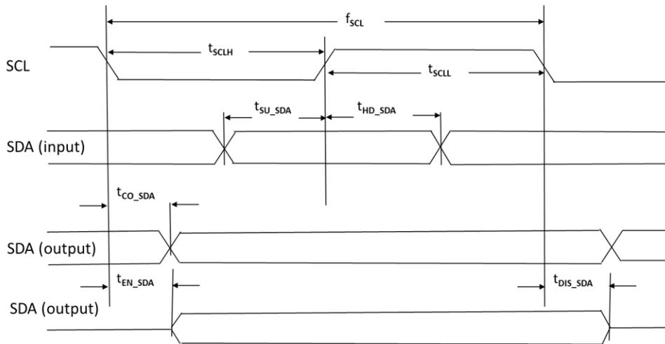
**Figure 3.20. I<sup>2</sup>C/I3C Configuration Timing**
