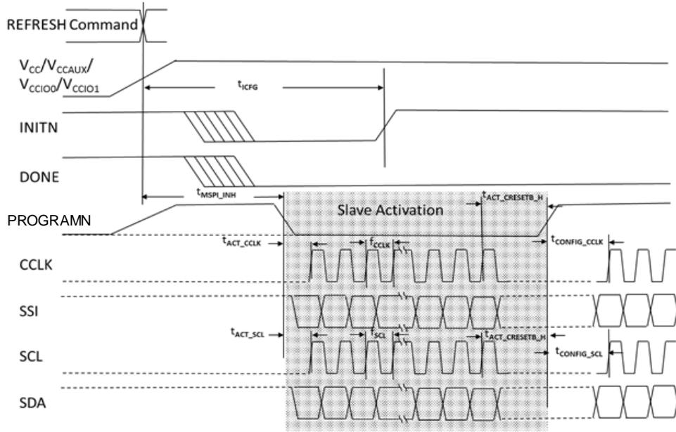
Figure 3.15. Slave SPI/I<sup>2</sup>C/I<sup>3</sup>C POR/REFRESH Timing
