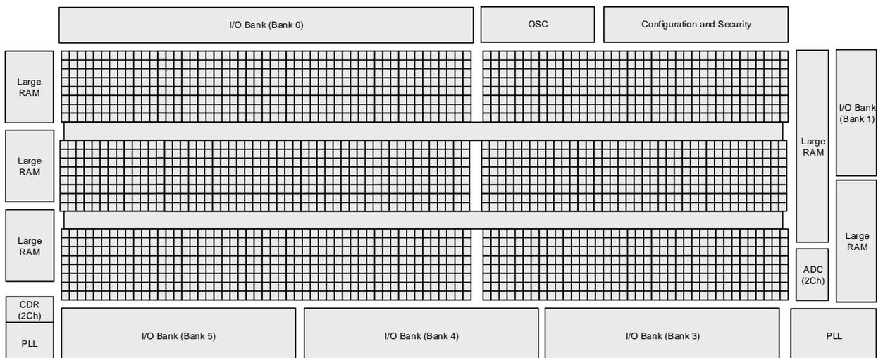
**Figure 2.2. Simplified Block Diagram, LFD2NX-17 Device (Top Level)**
