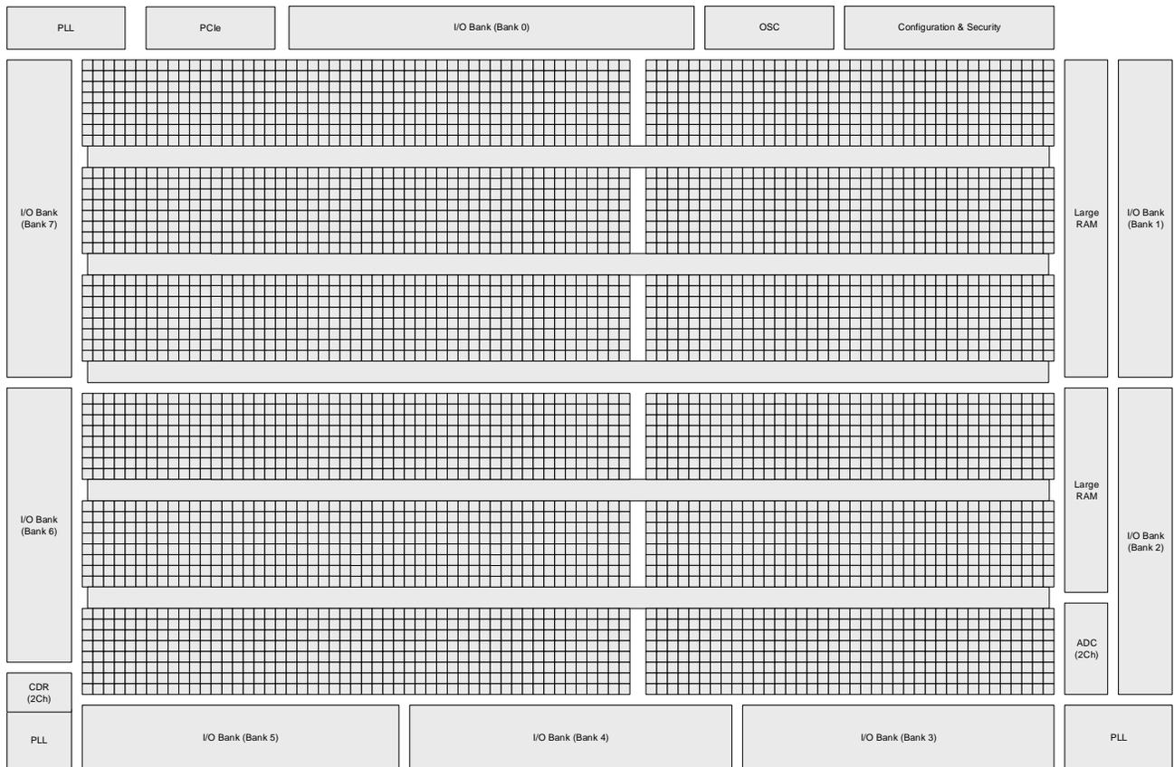
**Figure 2.1. Simplified Block Diagram, LFD2NX-40 Device (Top Level)**
