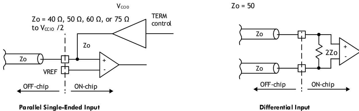
**Figure 3.1. On-Chip Termination**
