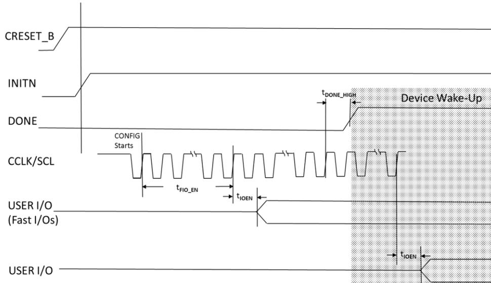
**Figure 3.22. Slave SPI/I<sup>2</sup>C/I<sup>3</sup>C Wake-Up Timing**
