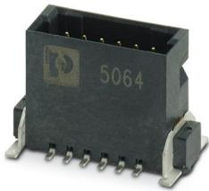
SMD male connector, nominal current: 1.4 A, Test voltage: 500 V AC, number of positions: 40, pitch: 1.27 mm, color: black, contact surface: Gold, contact connection type: Pin, mounting: SMD soldering
