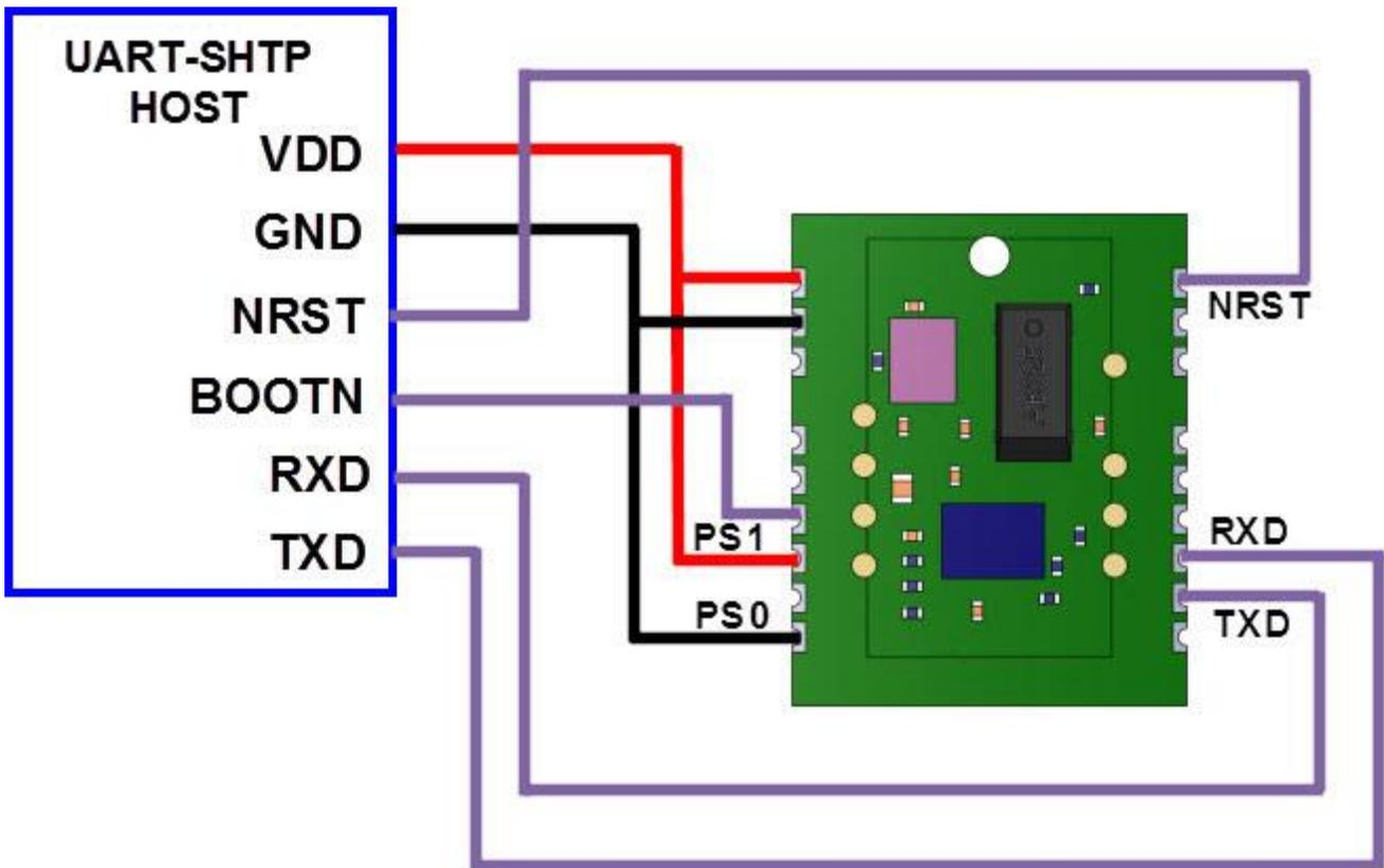
Figure 5: UART-SHTP Connection Example
