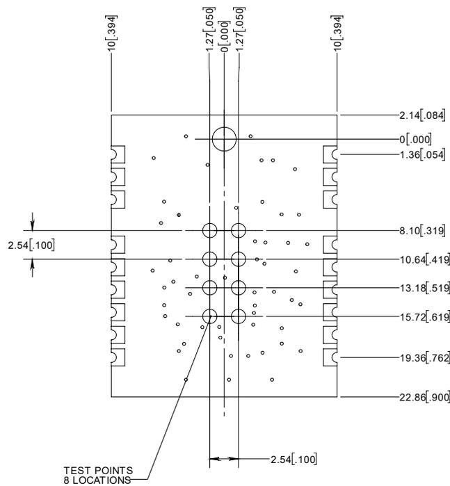
Figure 15: 18 pin module package outline (Bottom View)
