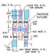
NOTES: 1. TRACE WIDTH IS SHOWN FOR ROGERS RO4350B WITH DIELECTRIC THICKNESS .020" ± .0015"; COPPER: 1/2 OZ. ON EACH SIDE. FOR OTHER MATERIALS TRACE WIDTH MAY NEED TO BE MODIFIED.
