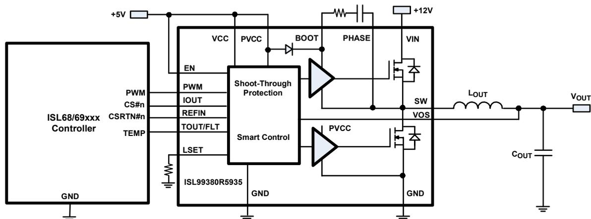
Figure 1. ISL99380R5935 Simplified Application Block Diagram
