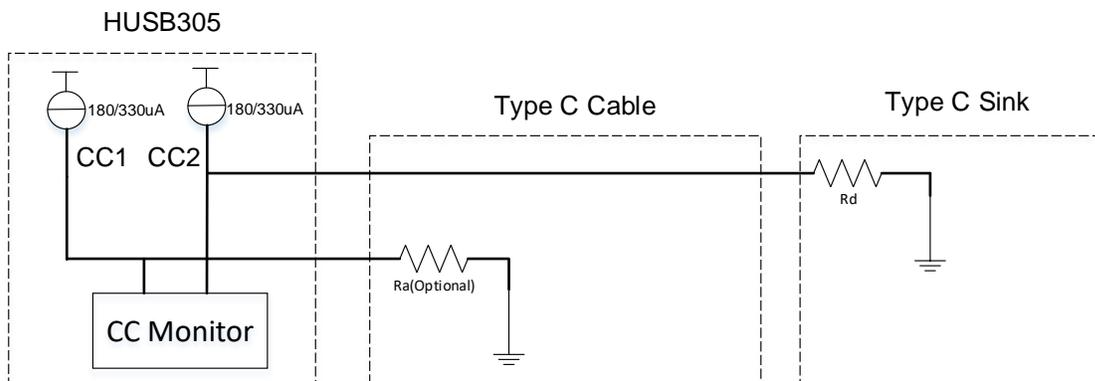
Figure 5. USB Type-C Source Connection with a Sink
