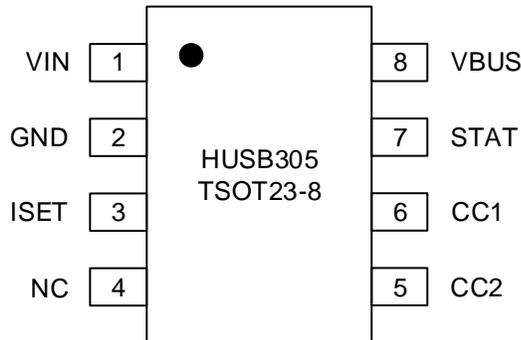
Figure 2. Pin Assignment
