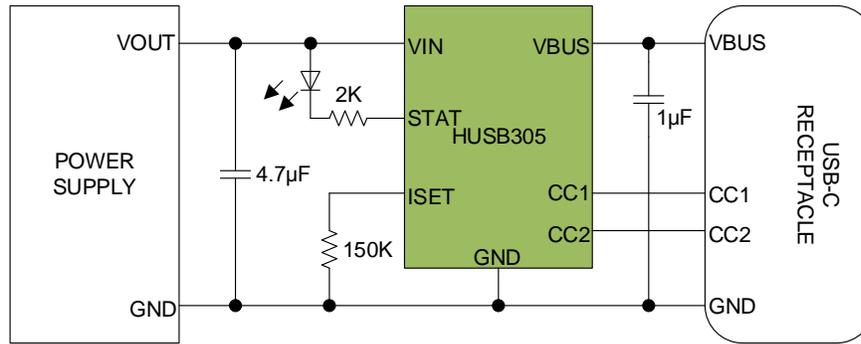
Figure 6. USB Type-C 5V3A Single Source Port
