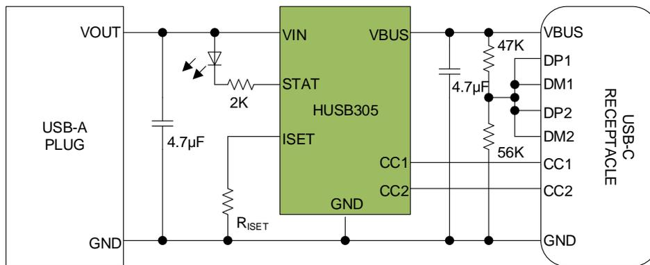
Figure 7. USB A to C Conversion Connector
