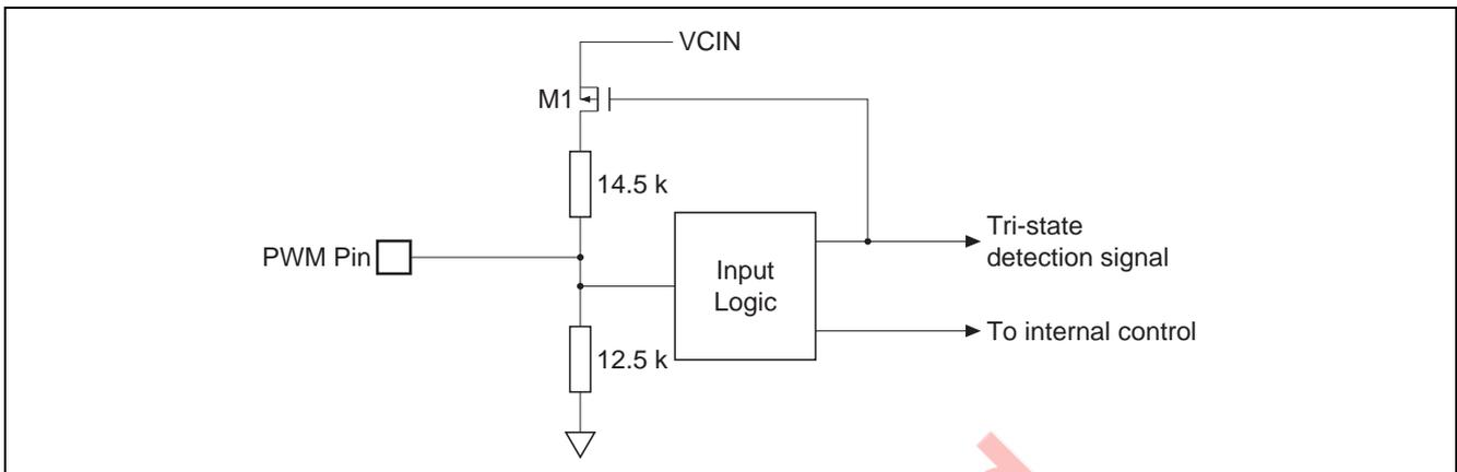
Figure 3 Equivalent Circuit for the PWM-pin Input
