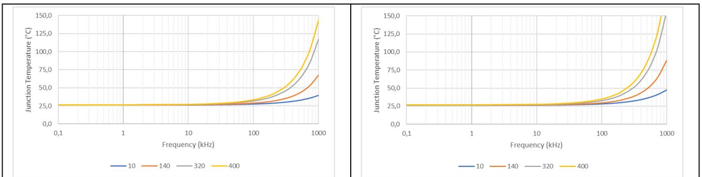
$R_{GATE}=10.2 \Omega$ ,  $V_{CC}=15 \text{ V}$ , CoolMOS™ IPS70R1K4P7S
