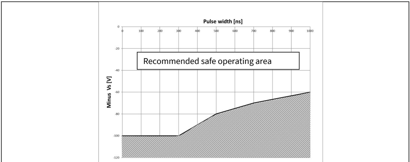
**Figure 19** Negative  $V_s$  transient SOA for 2ED2110S06M @  $V_{BS}=15$  V
