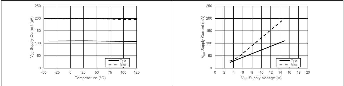
Figure 35 V<sub>DD</sub> Supply Current
