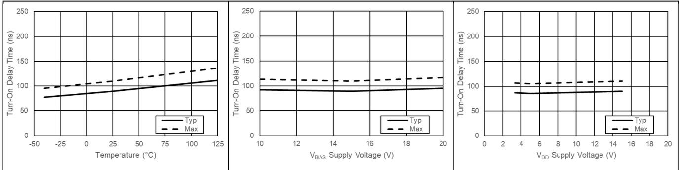
**Figure 24 Turn-On Delay Time**
