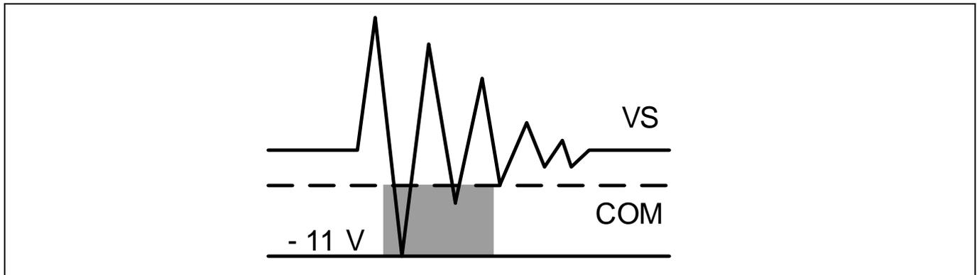
Figure 20 Headroom for HV level shifter data transmission
