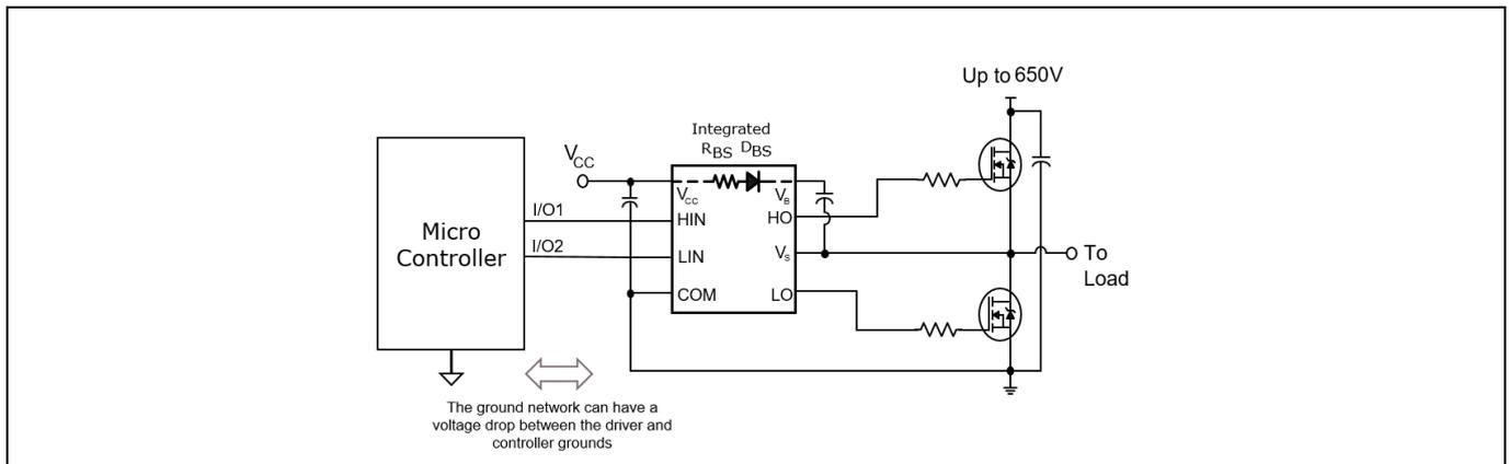
**Figure 15 Negative voltage tolerance on inputs of up to -5 V**
