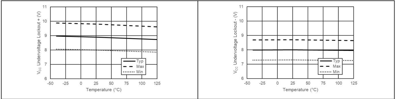
Figure 39 V<sub>CC</sub> Undervoltage Lockout
