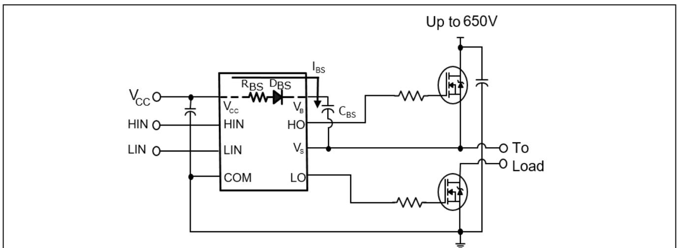
**Figure 14** Half bridge bootstrap circuit in 2ED2110S06M
