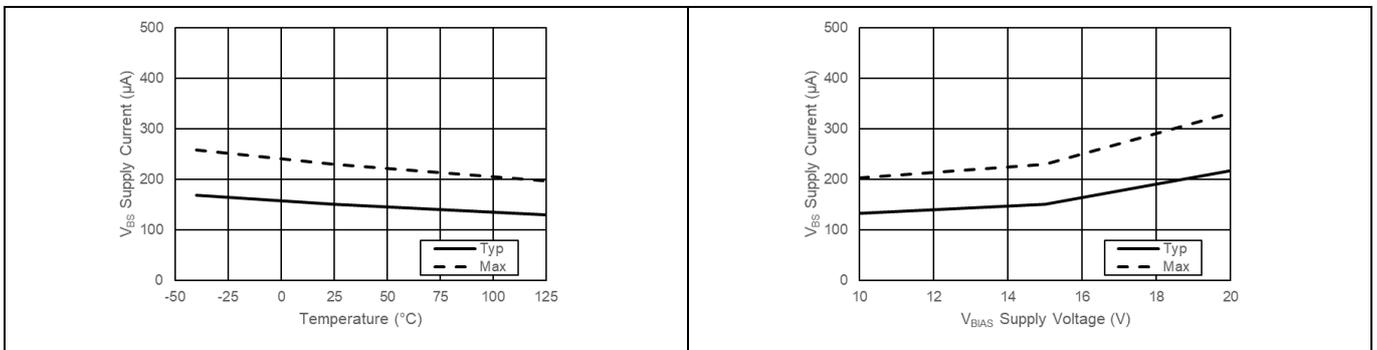
Figure 33 V<sub>BS</sub> Supply Current
