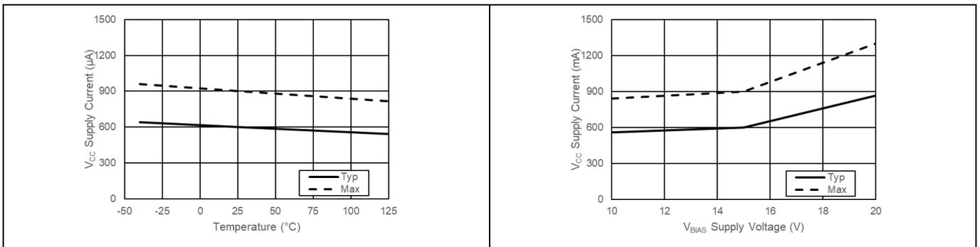
Figure 34 V<sub>CC</sub> Supply Current
