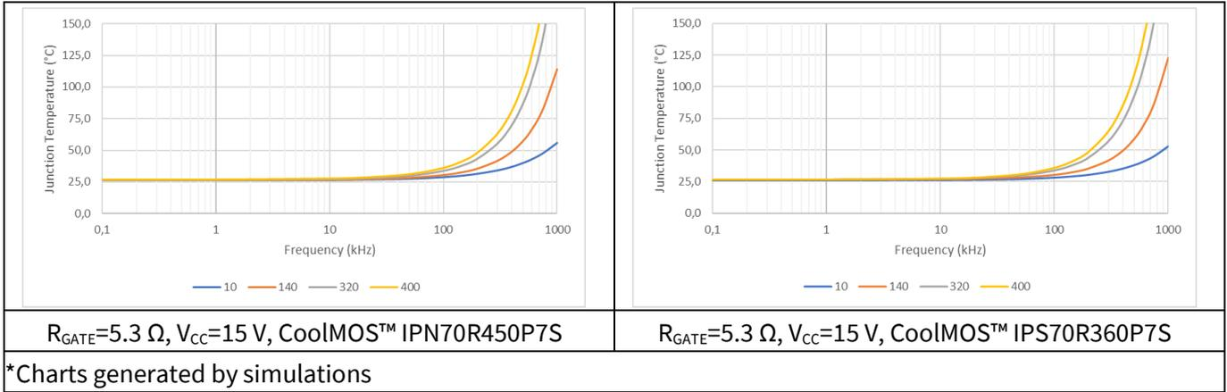
**Figure 43**  $T_j$  vs Frequency
