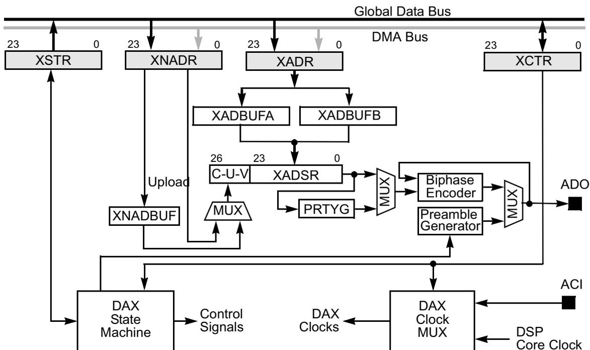
Figure 10-1 Digital Audio Transmitter (DAX) Block Diagram
