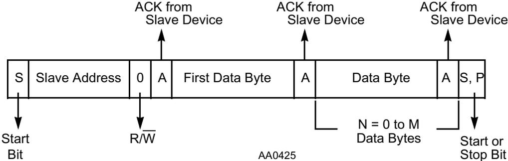
Figure 7-10 I<sup>2</sup>C Bus Protocol For Host Write Cycle
