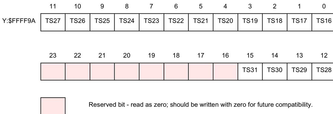
**Figure 9-12 TSMB\_1 Register**
