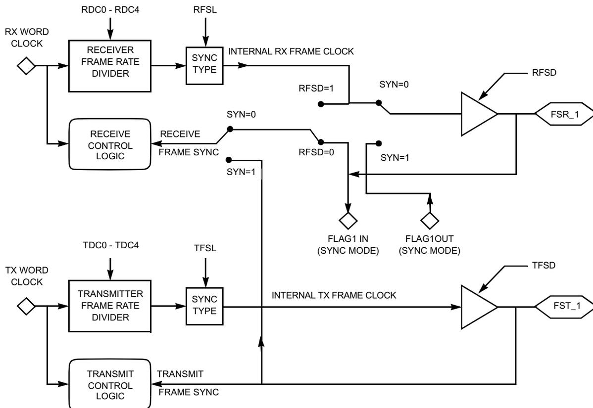
Figure 9-5 ESAI\_1 Frame Sync Generator Functional Block Diagram
