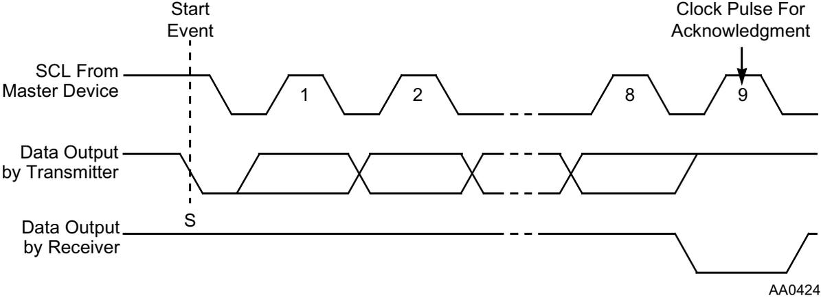
Figure 7-9 Acknowledgment on the I<sup>2</sup>C Bus
