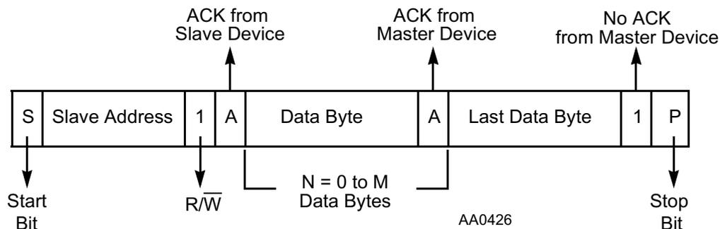
**Figure 7-11 I<sup>2</sup>C Bus Protocol For Host Read Cycle**
