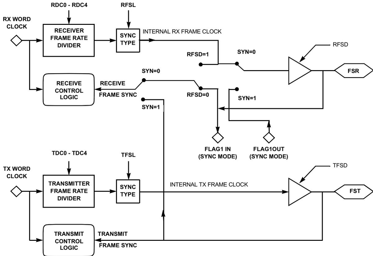
Figure 8-4 ESAI Frame Sync Generator Functional Block Diagram
