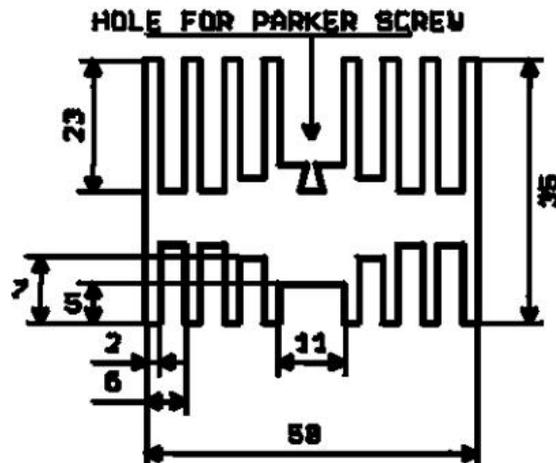
Figure 18: Example of heat-sink
