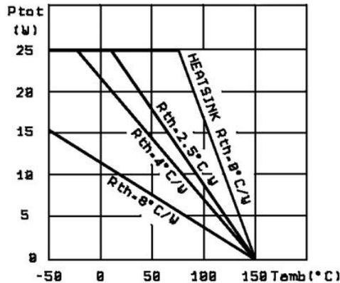
Figure 17: Maximum Allowable Power Dissipation vs. Ambient Temperature
