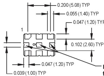
**NOTE: These 3 pads must be isolated from any traces or vias appearing beneath this port.**
