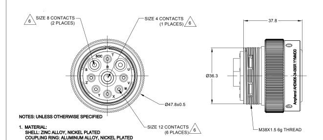
2. MODIFICATIONS: THREADED HOUSING; REDUCED DIA. SEAL
