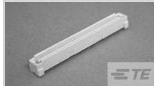
PCB Connector Assembly Type: **PCB Mount Header**PCB Mount Orientation: **Vertical**Connector System: **Board-to-Board**Number of Positions: **80**Centerline (Pitch): **.8 mm [.031 in]****Features****Product Type Features**
