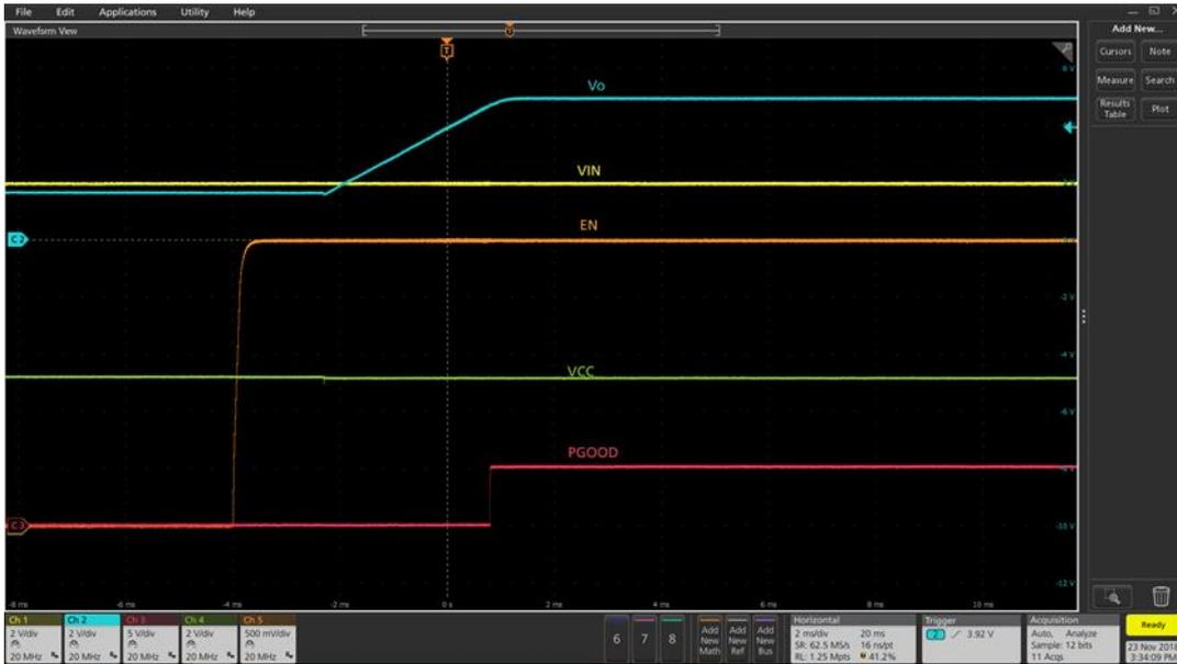
**Figure 20 Startup into pre-bias (Ch1:PV<sub>IN</sub>, Ch2: V<sub>OUT</sub>, Ch3: PGood, Ch4:V<sub>CC</sub>, Ch5: Enable)**
