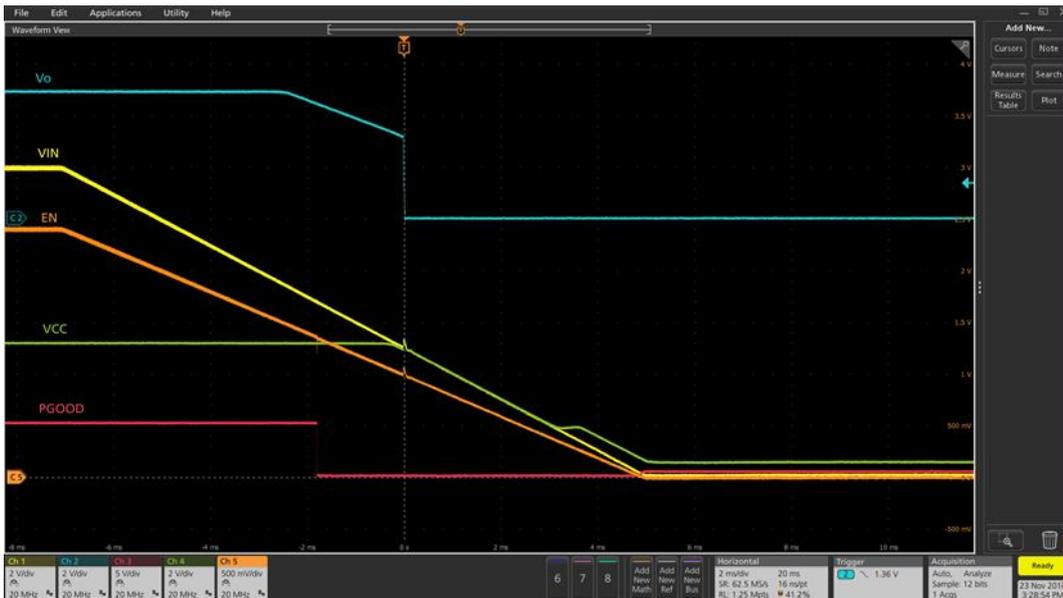
**Figure 18 Shutdown with Enable de-assertion at 3A load**
