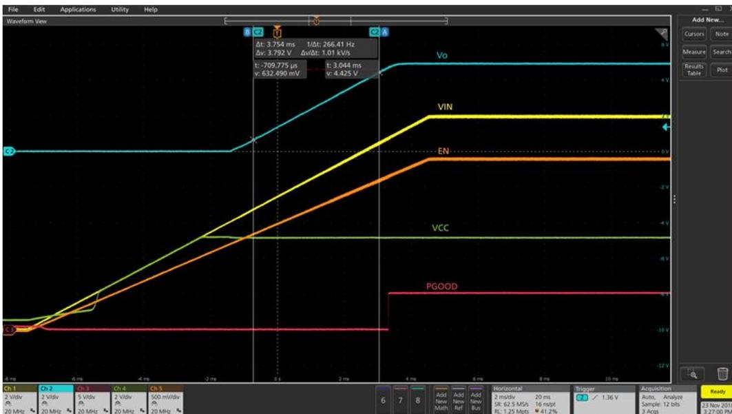
Figure 17 Startup with 3A load (Ch1:PV<sub>IN</sub>, Ch2: V<sub>OUT</sub>, Ch3: PGood, Ch4:V<sub>CC</sub>, Ch5: Enable)
