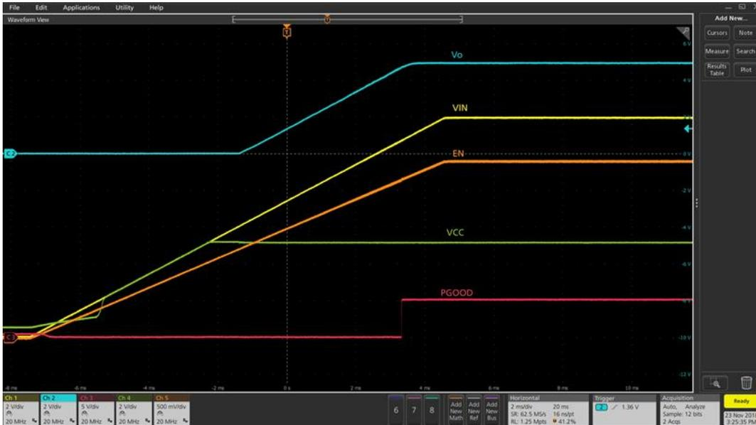
Figure 16 Startup with no load (Ch1:PV<sub>IN</sub>, Ch2: V<sub>OUT</sub>, Ch3: PGood, Ch4:V<sub>CC</sub>, Ch5: Enable)
