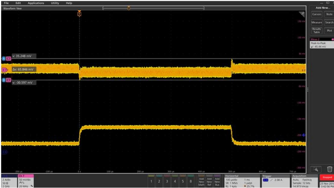
Figure 26 Transient response 1A to 3A (Ch6:Io, Ch2: VOUT), peak-peak deviation=66mV
