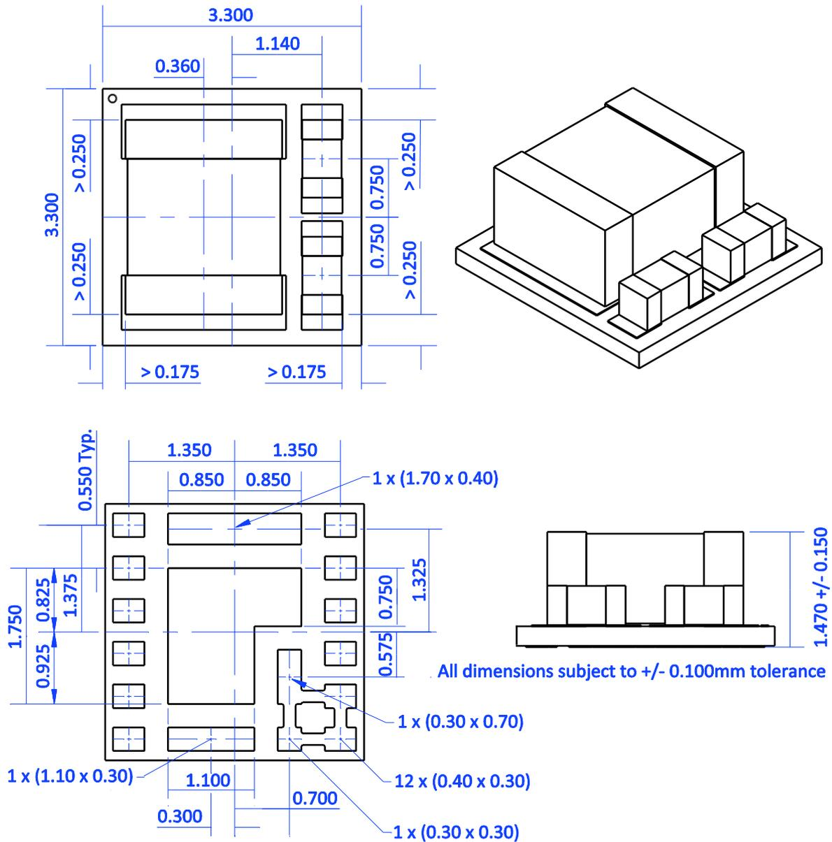
Figure 30 Dimensioned drawings
