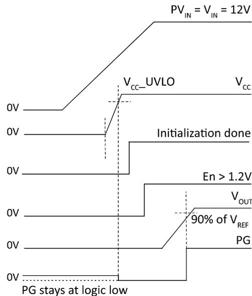
**Figure 10** Start-up: En pin asserted after PV<sub>IN</sub> and V<sub>IN</sub>, PG pin pulled up to an external supply
