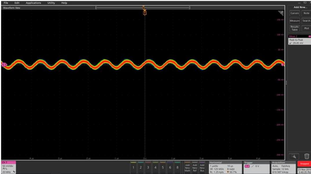
**Figure 24  $V_{OUT}$  ripple at 0A (Ch7:  $V_{out}$ ), Peak-Peak  $V_{OUT}$  ripple=30mV**
