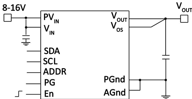
Figure 4 Typical applications circuit
