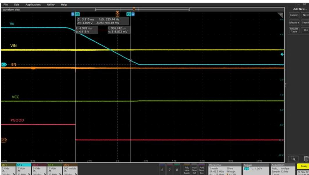
**Figure 19 Soft turn off at 3A load (Ch1:PV<sub>IN</sub>, Ch2: V<sub>OUT</sub>, Ch3: PGood, Ch4:V<sub>CC</sub>, Ch5: Enable)**
