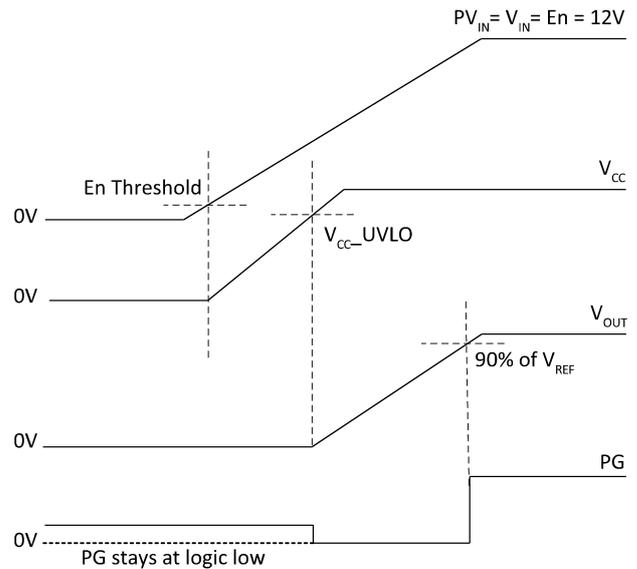
**Figure 9** Start-up: PV<sub>IN</sub>, V<sub>IN</sub> and En pins tied together, PG pin pulled up to an external supply
