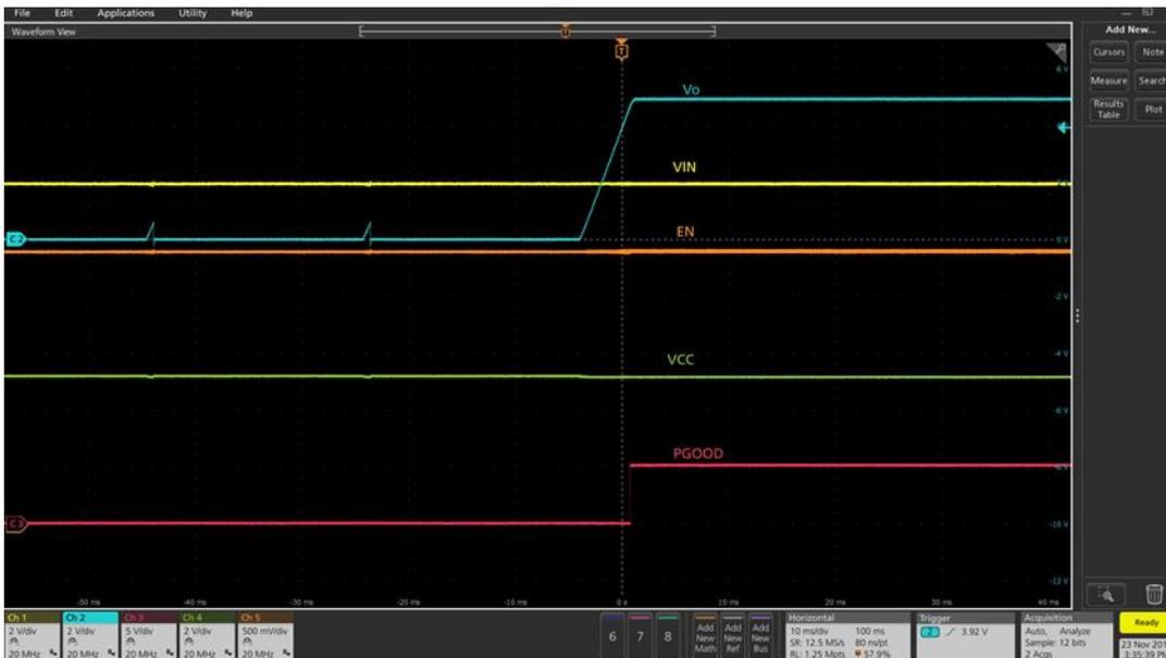
**Figure 21 Over-current protection and auto-recover to 3A (Ch1:PV<sub>IN</sub>, Ch2: V<sub>OUT</sub>, Ch3: PGood, Ch4:V<sub>CC</sub>, Ch5: Enable)**
