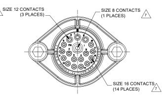
REDUCED DIA. WIRE SEAL SEALED PANEL MOUNT
