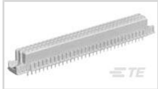
Connector & Housing Type: **Receptacle**Connector System: **Board-to-Board**Termination Post & Tail Length: **2.9 mm [.114 in]**Number of Positions: **96**Centerline (Pitch): **2.54 mm [.1 in]****Features****Product Type Features**
