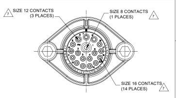
2. MODIFICATIONS: SMOOTH RING ADAPTER (SRA); STANDARD DIA. WIRE SEAL SEALED PANEL MOUNT
