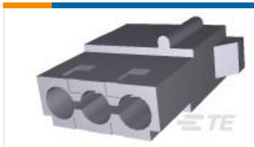
TE Part #1-175218-5 Contact: Component To Wire; 15A, 28-14 wire size
