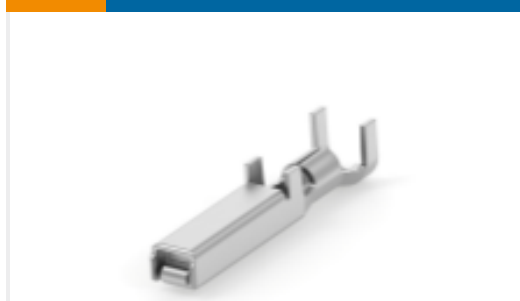
TE Part #1-175218-5 Contact: Component To Wire; 15A, 28-14 wire size
