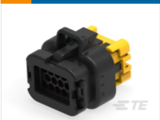
TE Part #2371883-1 14POS,AMPSEAL,SOC HSG ASSY,SLD, COD 1
