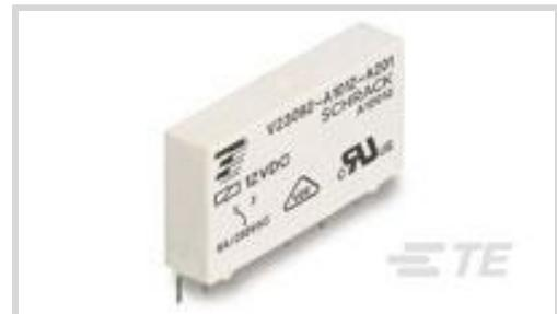
Power Relay Type: **Standard**Coil Magnetic System: **Monostable, DC**Coil Power Rating DC: **170 mW**Coil Resistance: **848 Ω**Coil Special Features: **UL Coil Insulation Class F**
