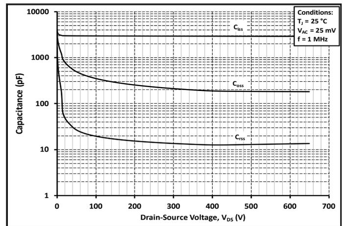
Figure 18. Capacitances vs. Drain-Source Voltage (0 - 650 V)
