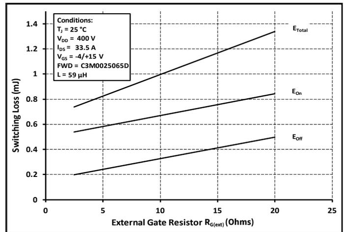
Figure 24. Clamped Inductive Switching Energy vs.  $R_{G(ext)}$
