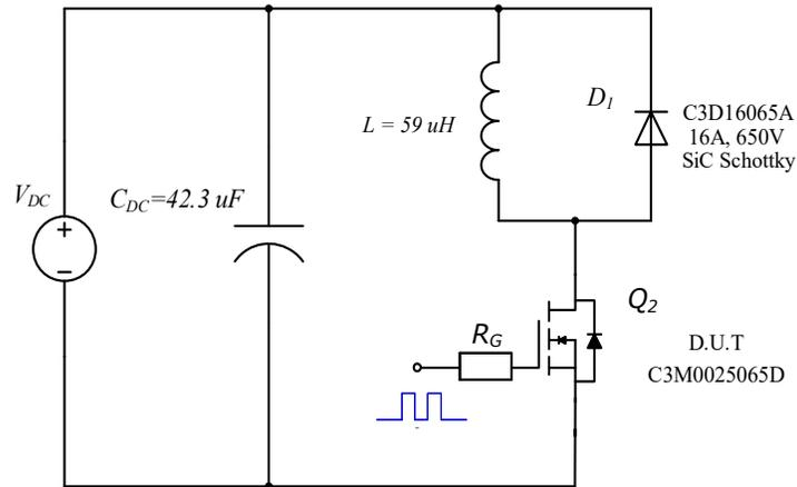
**Figure 27.** Clamped Inductive Switching Waveform Test Circuit
