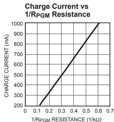
**Figure 3: Charge Current vs. 1/ $R_{PGM}$  Resistance**
