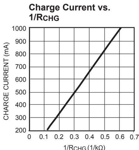
**Figure 3—Charge Current vs. 1/R<sub>CHG</sub> Resistance**
