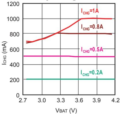
**$I_{CHG}$  Current vs Input Voltage**
