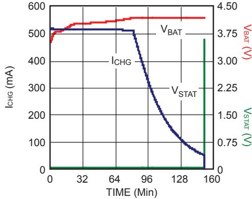
**Charge Current vs Battery Voltage**
