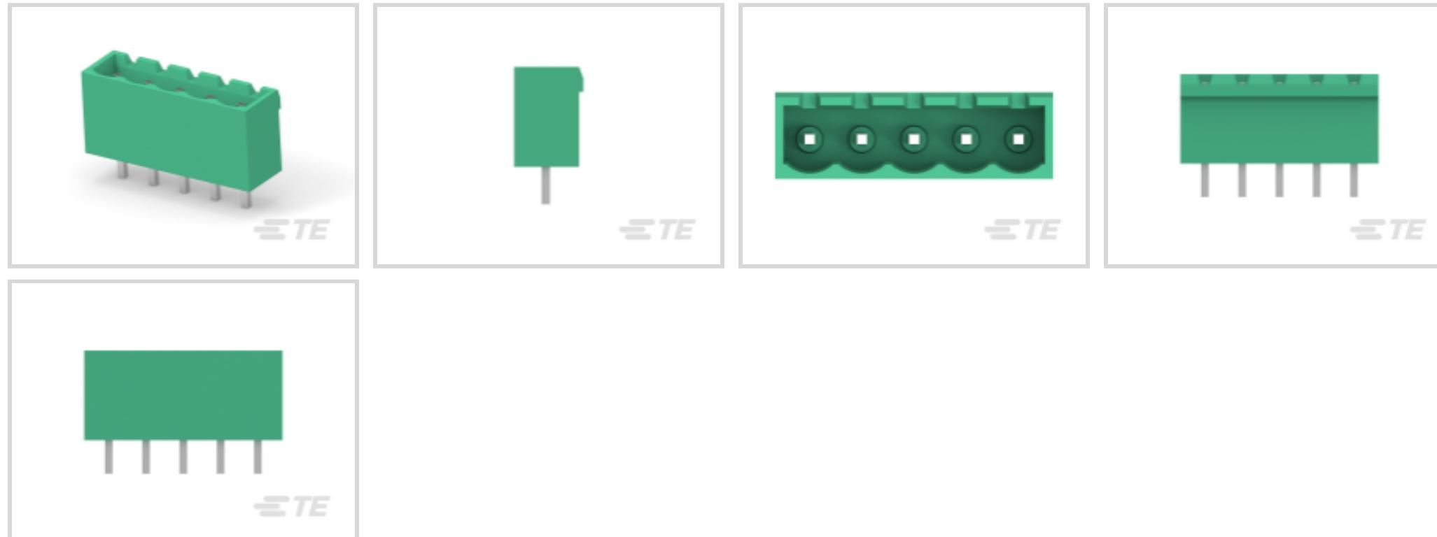
Terminal Block Connector Type: **Header**Connector System: **Wire-to-Board**Number of Positions: **5**Centerline (Pitch): **5 mm [.197 in]**Number of Rows: **1**
