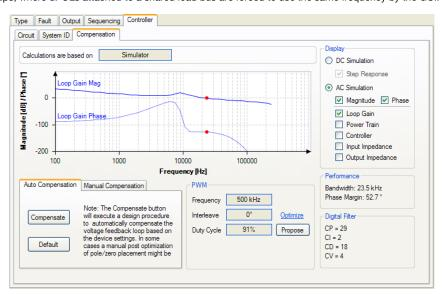
Figure 40. PWM Controller Window
