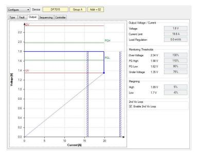
Figure 11. Output Configuration Window
