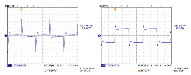
Figure 14. Transient Response without Optimal Voltage Positioning
