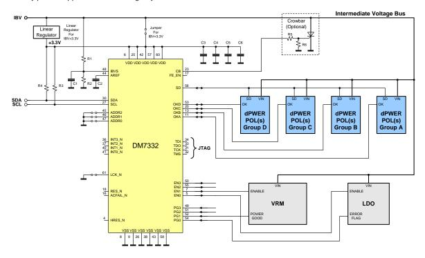
Figure 50. Multi-dPOL Power System Diagram
