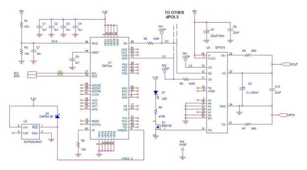
Figure 51. Typical Application with Digital Power Manager and I2C Interface
