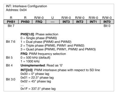
Figure 41. Interleave Configuration Register INT
