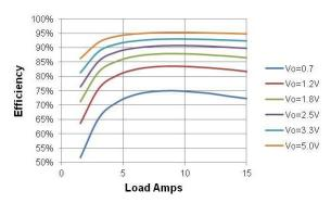
Figure 3. Efficiency vs. Output Voltage, lout=15A, Fsw=500kHz
