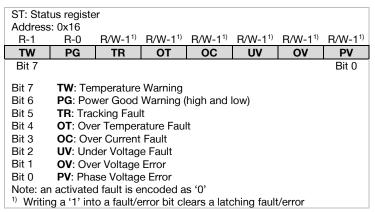
Figure 32. Protection Status Register ST
