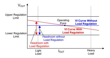
Figure 13. Concept of Optimal Voltage Positioning
