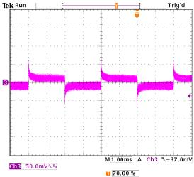
Figure 47. Transient Response with Regulation set to 0.0 mV/A
