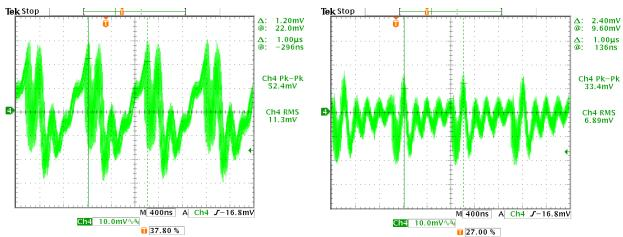
Figure 42. Input Voltage Noise, No Interleave
