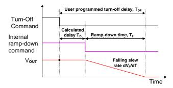
Figure 18. Relationship between Turn-Off Delay and Falling Slew Rate
