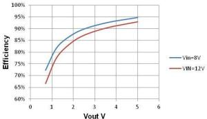
Figure 5. Efficiency vs. Load. Vin=12V, Fsw=1MHz
