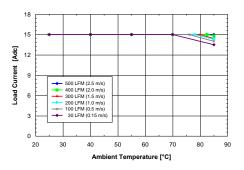
Figure 9. Thermal Derating Curves. Vin=12V, Vout=5.0V, Fsw=500kHz
