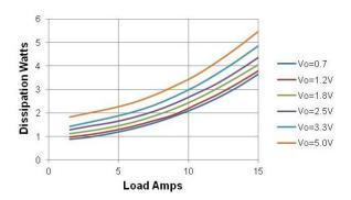
Figure 7. Dissipation vs Load, Vin=12V, Fsw=500KHz
