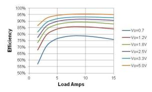
Figure 1. Efficiency vs. Load. Vin=8V, Fsw=500kHz
