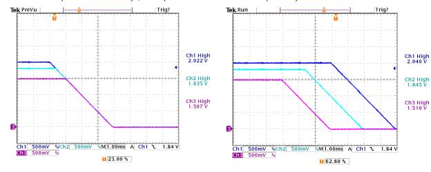
Figure 26. Tracking Turn-Off. Falling Slew Rate is programmed at 0.5V/ms.
