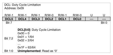
Figure 46. Duty Cycle Limit Register
