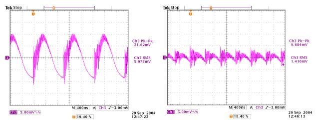
Figure 44. Output Voltage Noise, Full Load, No Interleave
