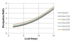
Figure 8. Dissipation vs Load, Vin=12V, Fsw=1MHz
