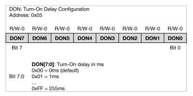
Figure 17. Turn-On Delay Register DON
