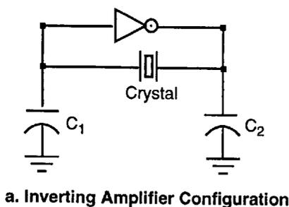
a. Inverting Amplifier Configuration
