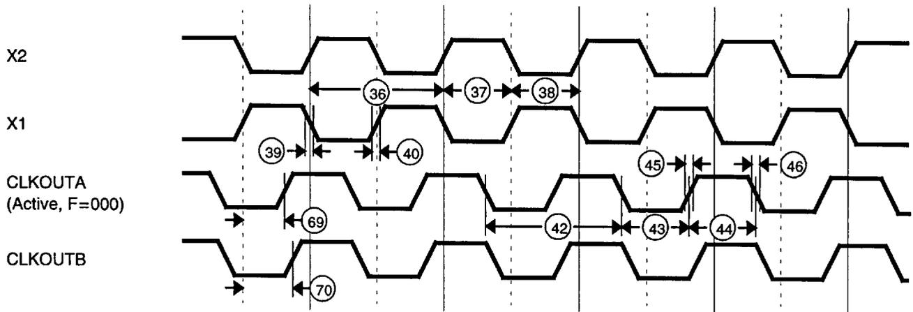
**Clock Waveforms—Power-Save Mode**
