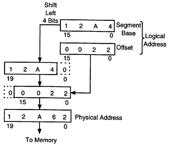
**Figure 2. Two-Component Address**
