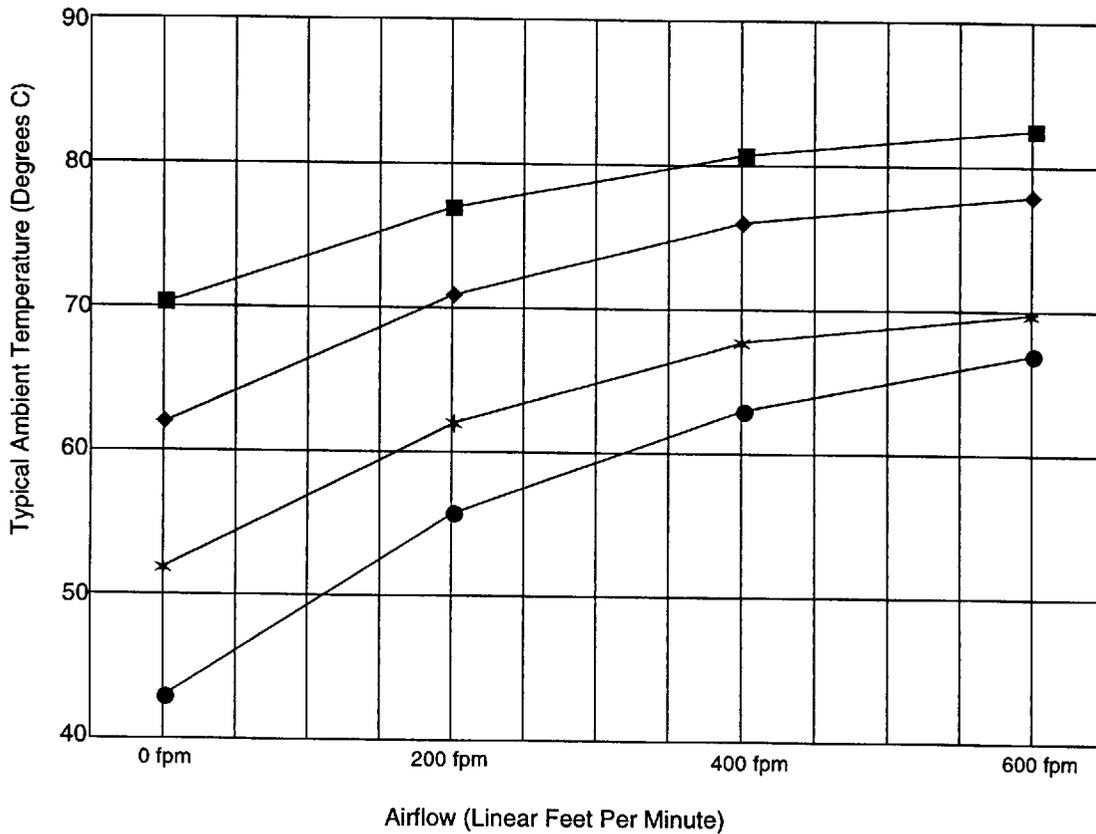
**Figure 18. Typical Ambient Temperatures for TQFP with 2-Layer Board**
