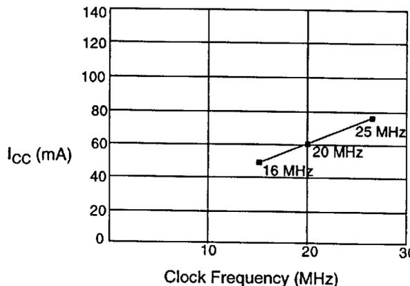
**Figure 13. Typical  $I_{CC}$  Versus Frequency for the Am186EMLV and Am188EMLV**
