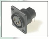
ACF / PC 3 Pin right angle PCB mounting Female XLR with counter sunk mounting holes for M3 screw fixing. XACF / PC has non counter sunk mounting holes for self-tap screw fixing. Nickel Silver plated Brass contacts.
