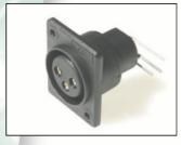
XACFR / PC 3 Pin horizontal lateral right PCB mounting Female XLR with self-tap screw fixing. Vertical PCB mounting versions ACF / PCS and XACF / PCS available. Nickel Silver plated Brass contacts.
