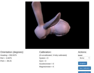
If you move the BNO055 sensor you should see the 3D model move too. However when the demo first runs the sensor will be uncalibrated and likely not providing good orientation data. Follow the next section to learn how to calibrate the sensor.
