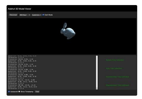
That raw data is all fine and good, but we want to see what they mean in 3D space, right? Traditionally, a Processing sketch would be used to read the serial data and convert it to a 3D rotation - but thanks to Web Serial API we can use any Chrome browser - a lot easier than installing Processing! ()
