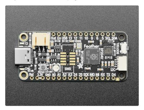
As of November 28, 2022 – we've updated this Feather with a right-angle tactile button for the Bootloader switch, so that you can press it even when a 'wing is on the Feather. We have also connected the boot button to GPIO #4 so it can be used as a user-input button.
