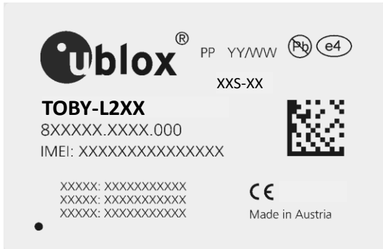
Figure 7: Example of TOBY-L2 series module label
