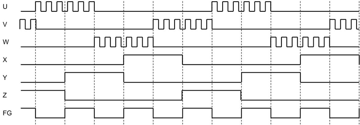
\*: When CW/CCW = Low, inverted Hall signals put the TB6584AFNG in 120 commutation mode with a lead angle of 0° (reverse rotation).
