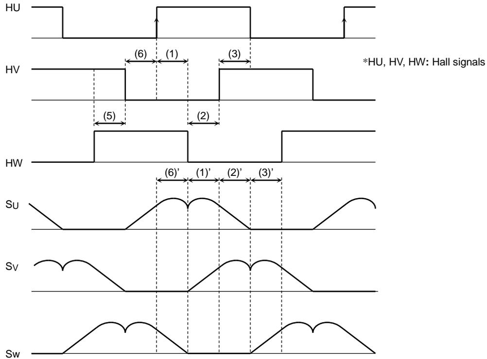
In the above diagram, the modulated waveforms have an interval ((1)') equal to the interval of 1/32 between a rising edge of HU to a falling edge of HW ((1)). And the modulated waveforms have an interval ((2)') equal to the interval of 1/32 between a falling edge of HW to a rising edge of HV ((2)). If there is not an HU rising edge before 32 ticks ends, (2)' becomes equal to (1)' until the next rising edge of HU.
