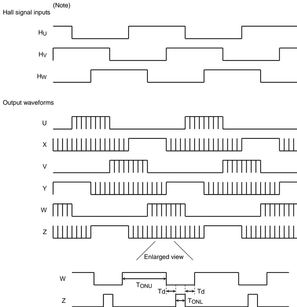
Note: Square waveforms are used in the above diagram for the sake of simplicity.
