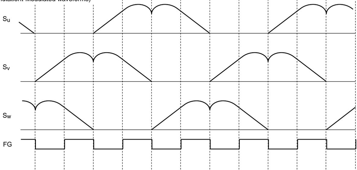
\*: When the Hall input frequency is equal to or greater than approximately 5.7 Hz (@ f<sub>osc</sub> = 4.5 MHz), lead angle control is activated according the LA input.
