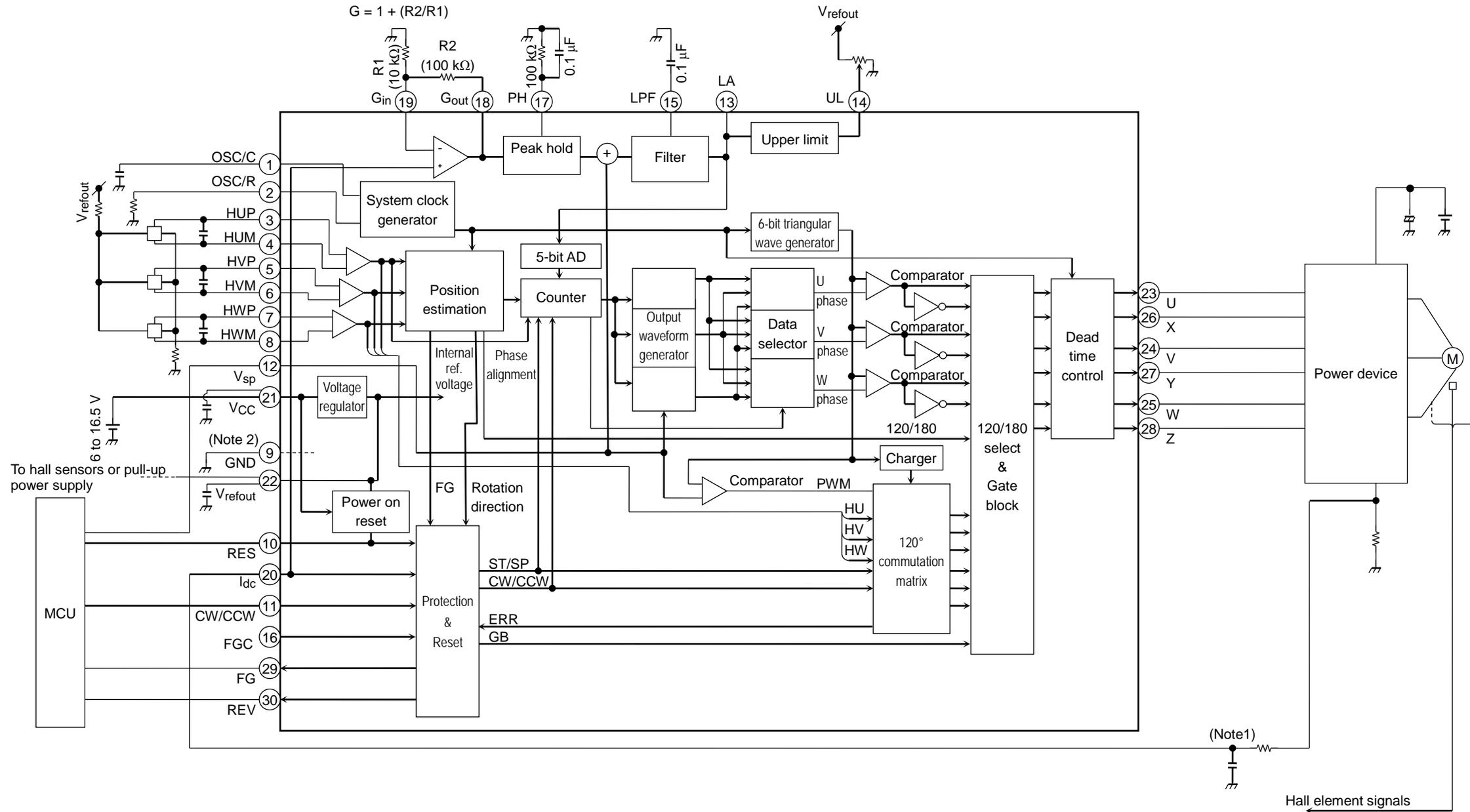
Note 1: Connect to ground as necessary to prevent IC malfunction due to noise.
