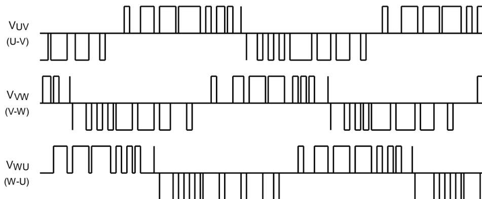
In sine-wave drive mode, the amplitude of the modulated signals varies with the  $V_{sp}$  voltage, and the motor speed changes with the conduction duty cycle of the output waveforms. (See the sine-wave drive mode diagram on page 15.)
