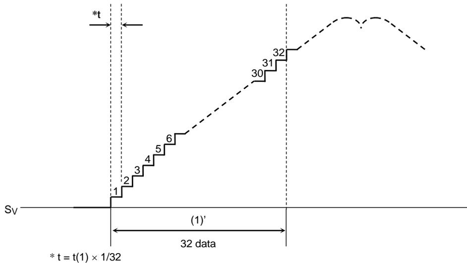
Phase of data and modulated waveform is adjusted for every zero cross of position detecting signal.
