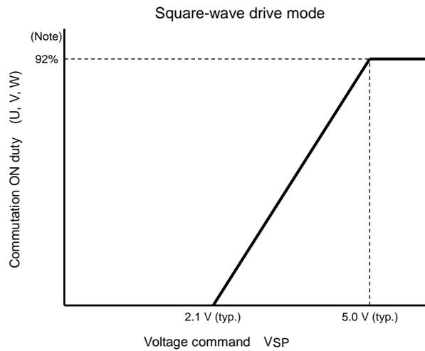
Note: The conduction period is reduced by the dead time.  $(\text{carrier period} \times 92\% - T_d \times 2)$
