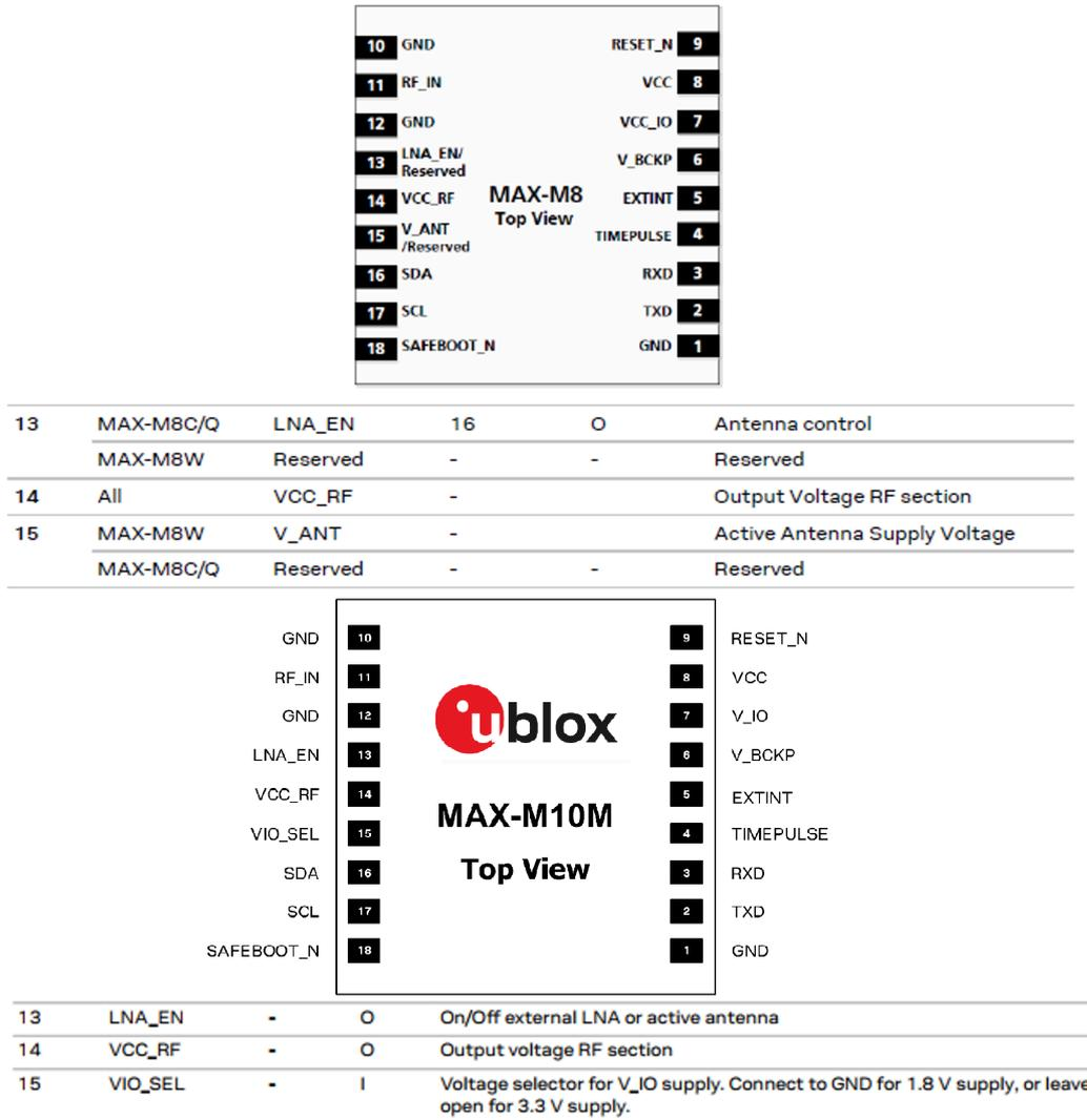
Figure 35: MAX-M8 vs. MAX-M10M comparison (pin 13 - 15)
