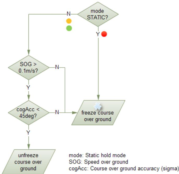
Figure 5: Flowchart of course over ground freezing
