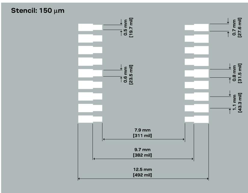
Figure 31: Recommended paste mask pattern for MAX-M10M
