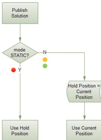
Figure 3: Position output in static hold mode
