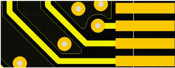
**Figure 28: GND stub ended with a via**
