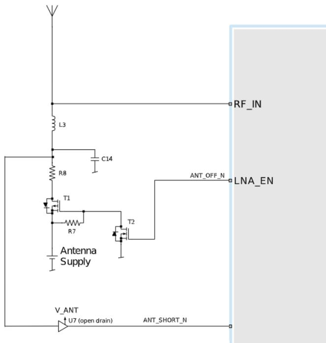
**Figure 11: MAX-M10M two-pin antenna supervisor**
