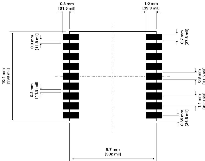
Figure 30: Recommended copper land and solder mask opening for MAX-M10M
