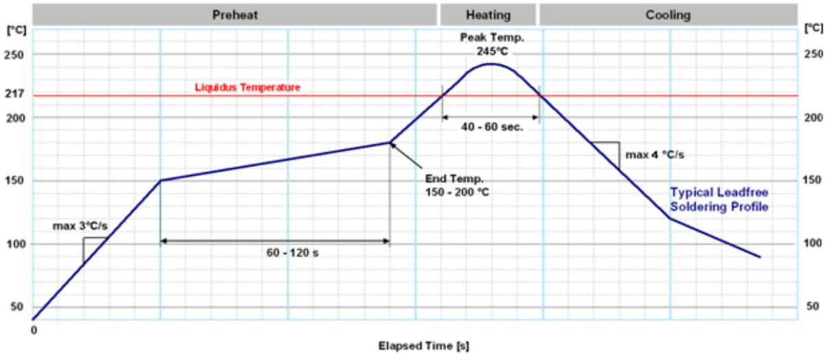
Figure 34: Soldering profile
