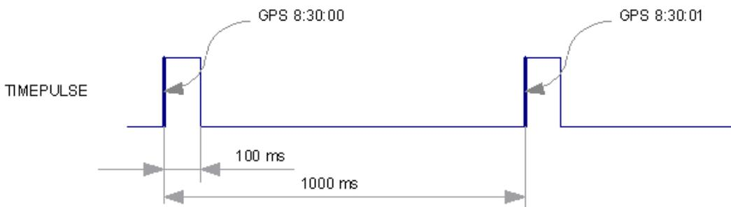
Figure 18: Time pulse signal with the example parameters
