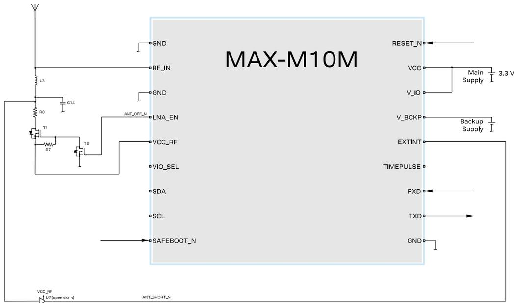
**Figure 38: 2-pin antenna supervisor design**
