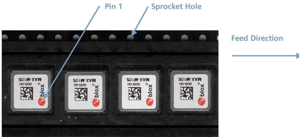
Figure 32: Orientation of the components on the tape
