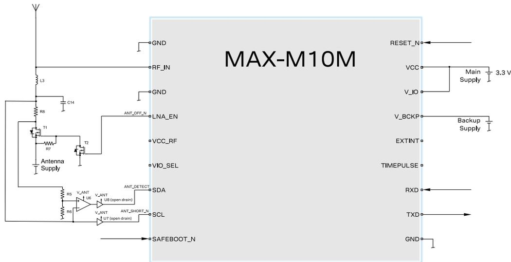
**Figure 39: 3-pin antenna supervisor design**
