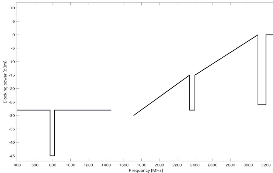
Figure 26: MAX-M10M out-of-band immunity level at 400 - 1460 MHz and 1710 - 3300 MHz for the normal-gain mode (default). Preliminary data subject to change.
