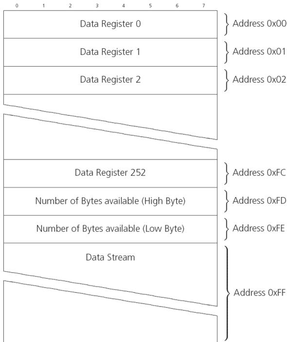
**Figure 6: I2C register layout**
