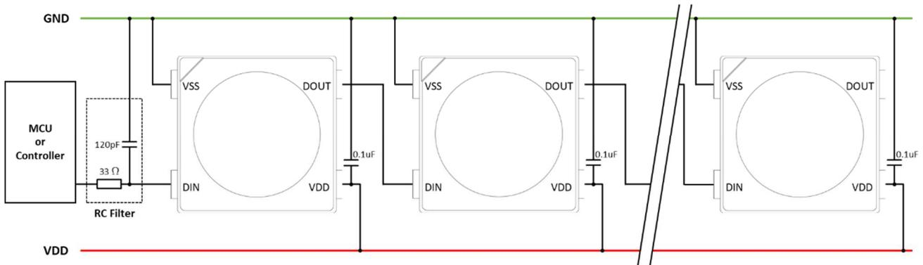
Cascading connection for normal driver IC embedded LEDs is shown. The data signal is transmitted one-by-one. The output of the previous one is connected to the input of the next one. As for the power positive and negative, all LED positives should be connected to VDD and all LED negatives should be connected to ground.
