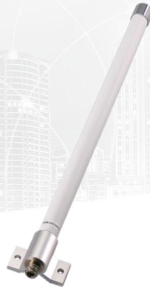
The Barracuda OMB.242.08F21 has been designed to provide long distance coverage at the 2.4-2.5GHz Wi-Fi band. The OMB.242 is a fiberglass robust outdoor antenna for use where an omnidirectional radiation pattern is required. The base is aluminum - meaning it is resistant to rusting. The fiberglass enclosure is UV coated making this antenna suitable for the harshest outdoor environments. The Barracuda is IP65 rated and can be mounted in areas where installation may be difficult.
