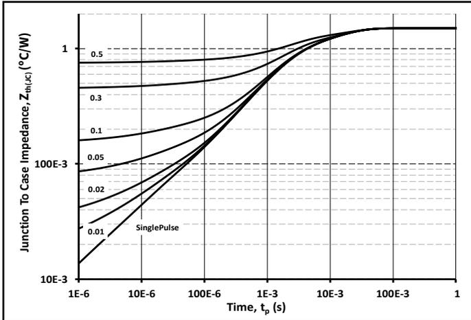
Figure 21. Transient Thermal Impedance (Junction - Case)
