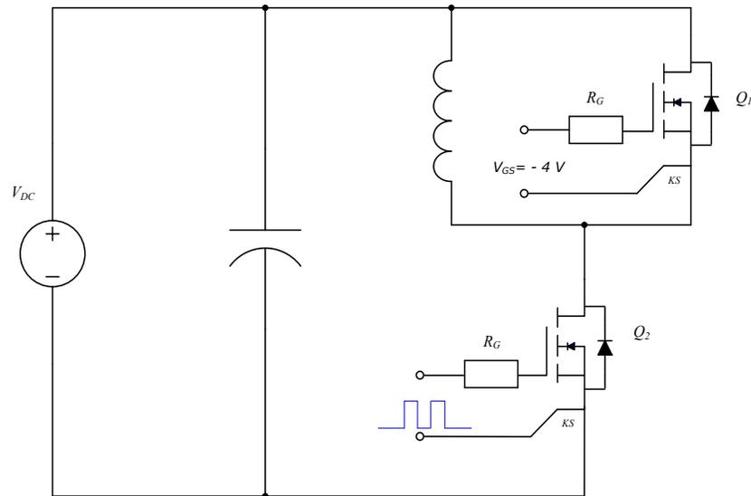
**Figure 29.** Clamped Inductive Switching
