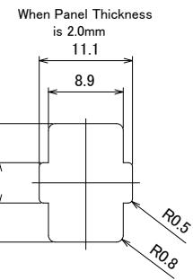
A chamfer of C0.1 is required in order to prevent scrapping to the cover case during panel installation. Number of panel installation can be used up to 10 times.
