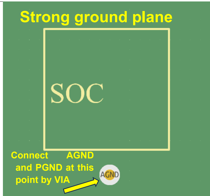
Figure 2: Suitable way of connecting AGND and PGND (at Inner Layer)
